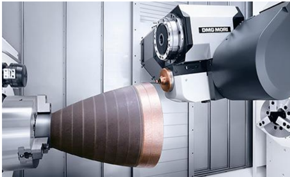
Figure 1. Deposition of a nozzle for a rocket engine made of stainless steel (X5CrNiMo17-12-2): \varnothing 450 \times 470 mm, approx. 10 h machining time incl. 6-sided turn & mill complete machining. [1]
