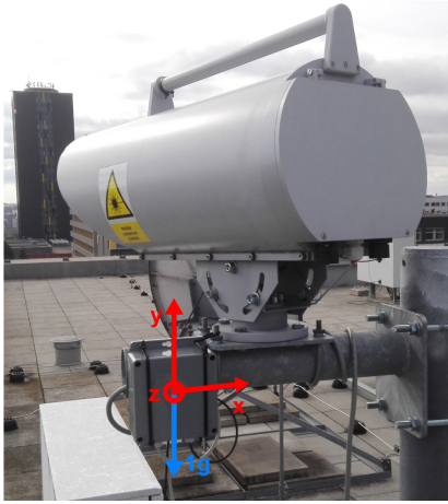
Fig. 2. Prototype of device for vibration measurement installed on FSO fixture.
