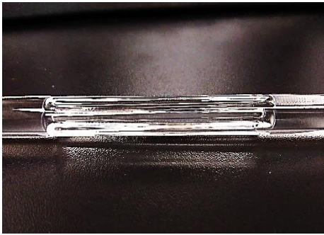
Fig. 2. Real image of thermally shaping optical fiber preform based CO2 laser.
