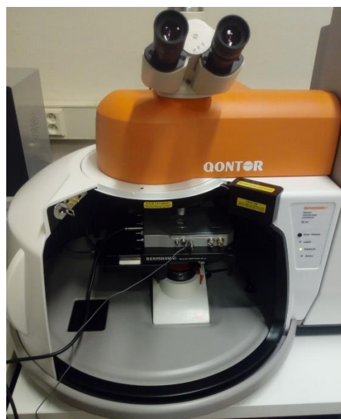
Fig. 1. The LINKAM chamber with embedded heater inside the Raman spectrometer.
