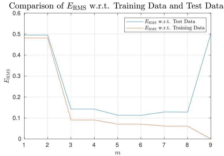
Figure 2.4: Figure compares calculated E_{\text{RMS}} error with respect to training data and test data sets; with polynomial of the ninth order the machine learns to perfectly fit the training data but gives very poor result to fit the test data.
