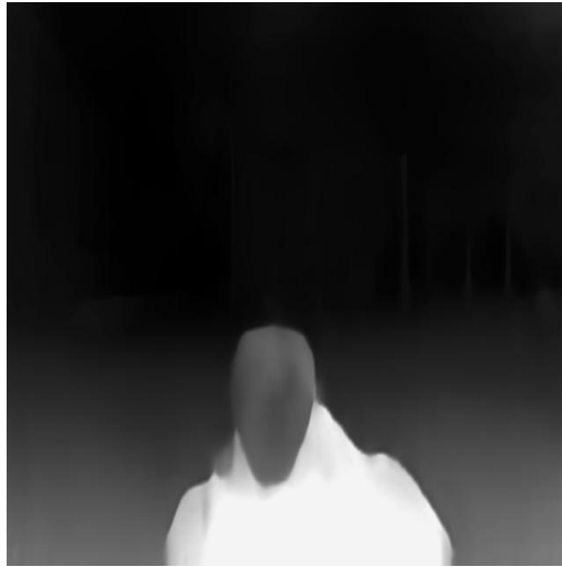
Figure 5.6: Example of resulted depth image processed with monodepth2 when converted to grayscale
