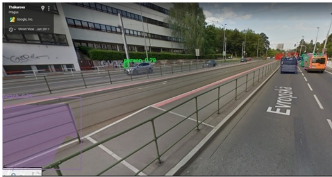
Figure 7.2: Misclassification of the grill (purple mask) as the bench with confidence score of 0.97
