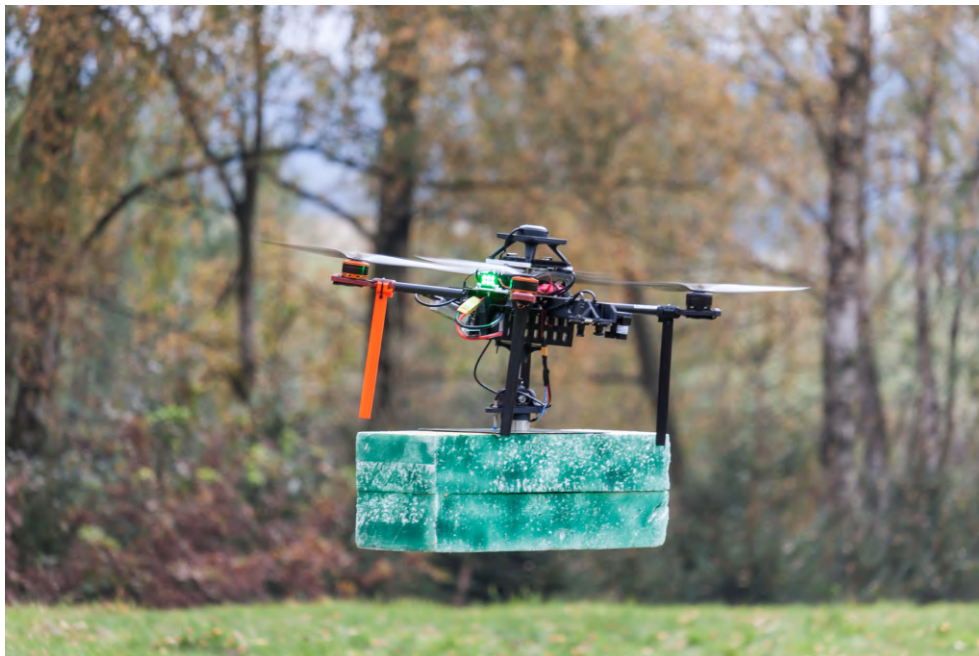
(b) Proposed gripper grasping a 1.6 kg brick
