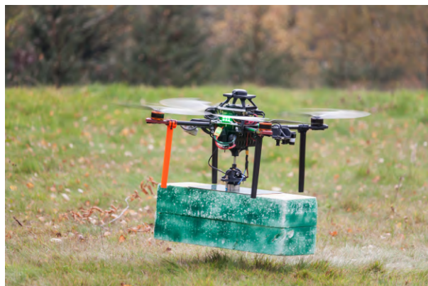
(a) The UAV hovers while placing the green brick
