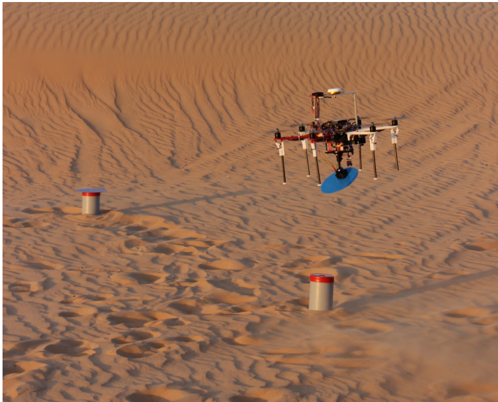
(a) Previously used EPM gripper grasping a 0.5 kg metal disk
