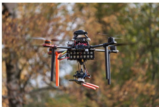
(c) UAV grasps pliers showing the versatility of the gripper
