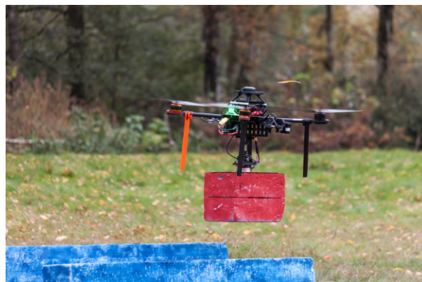
(b) UAV flies above the wall with the red brick
