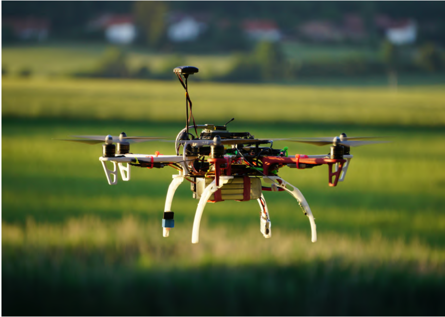
Figure 1.1: Example of a UAV with onboard instruments, GPS antenna and battery
