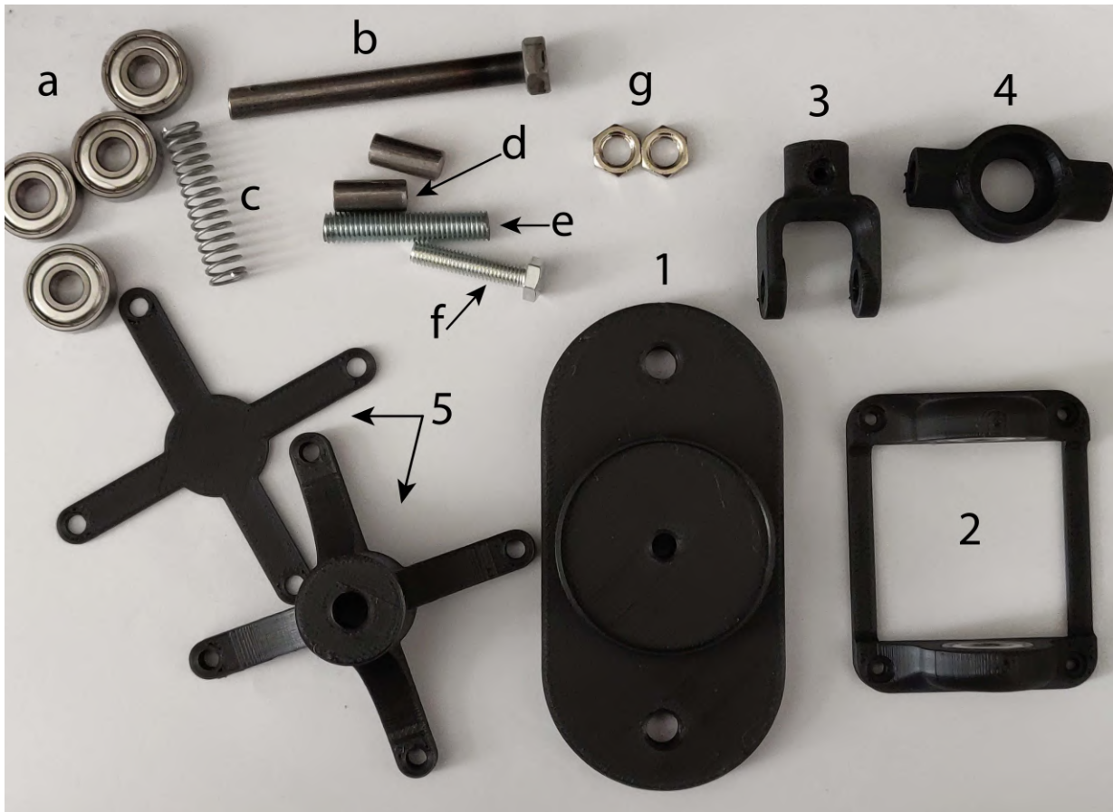
Figure 3.8: All mechanical components of the gripper
