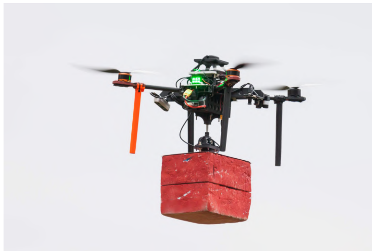
(a) UAV transporting red brick
