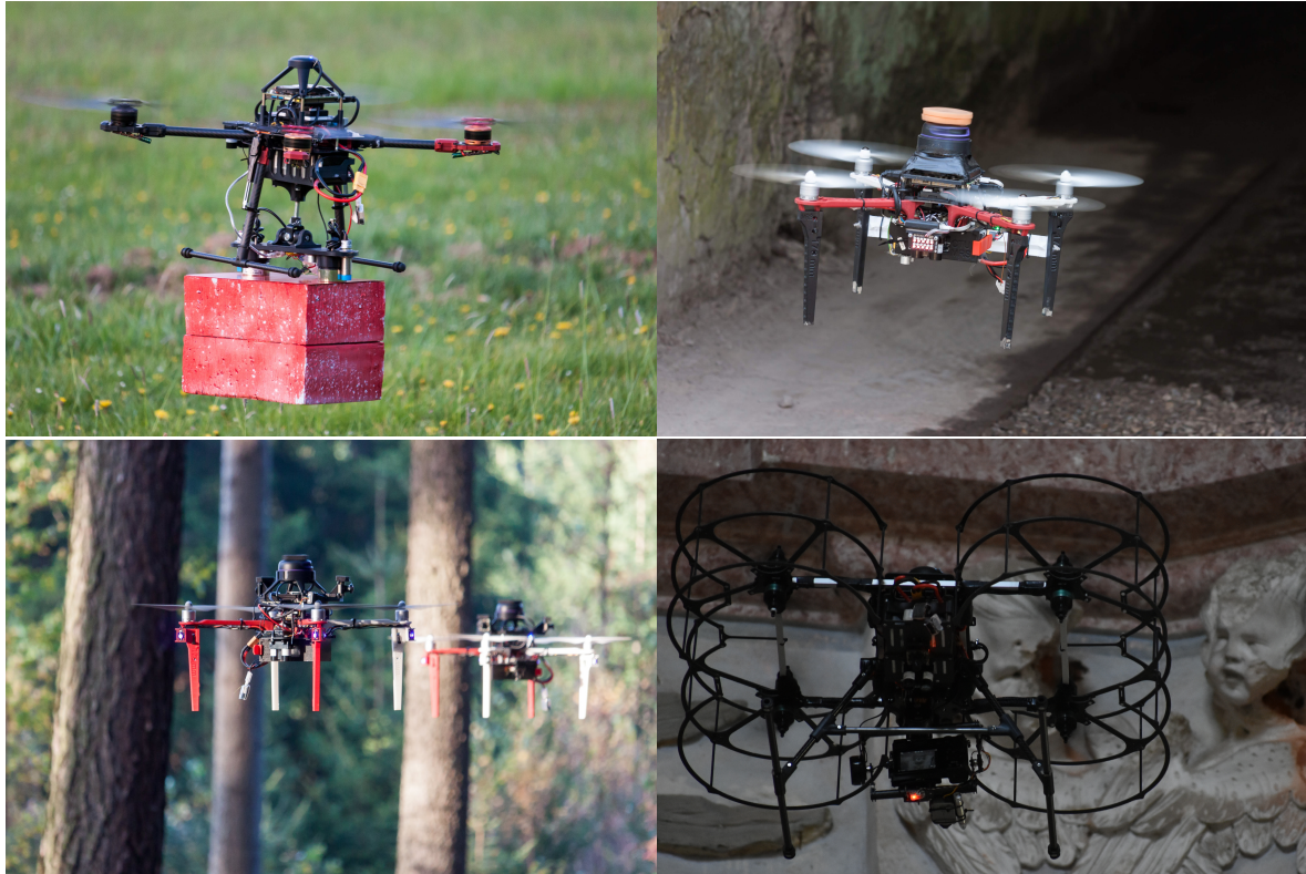
Figure 1.1: Examples of various UAV applications. The photo at the top left corner shows the magnetic brick holder attached to the UAV - scenario for MBZIRC 2020. At the top right corner is a UAV during the DARPA challenge in August 2019 [9]. At the bottom left corner shows the swarm of two UAVs in the forest during experiments with UVDAR [3]. In the bottom right corner is the UAV during church inspection [10].
