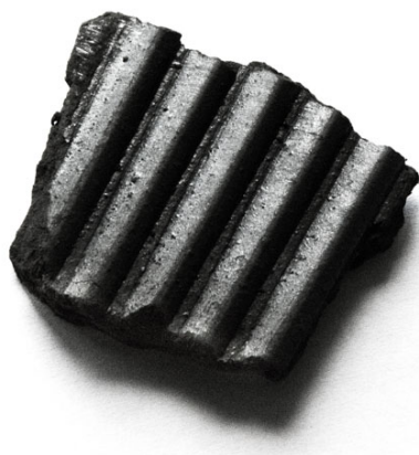
FIGURE 5. Profiled strip of experimental material from compaction process.
