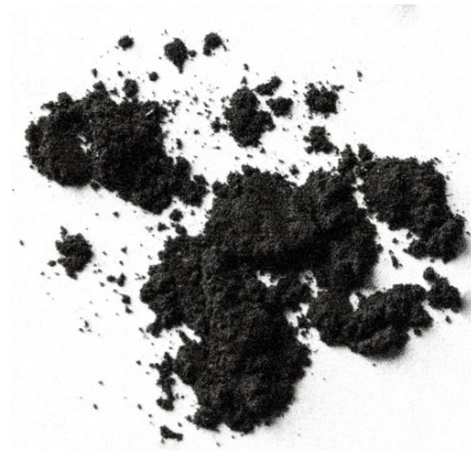
FIGURE 1. Powder from brake lining production.
