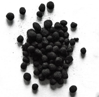
FIGURE 9. Final product produced by tumbling granulation process.
