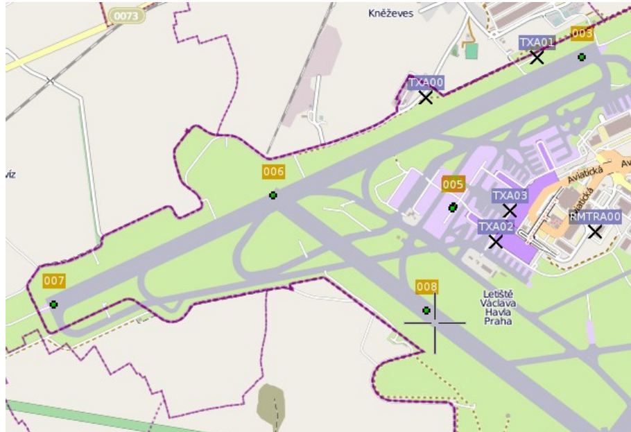
Figure 8.16: Situation plan of the Vaclav Havel Airport Prague with view to positions of transmitters (TXAxx) and measured points (00x) (shown on map layer of OSM maps)
