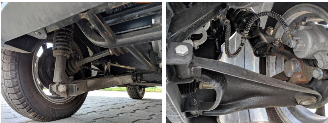
Figure 8 - Jiayuan City Spirit, left: rear left trailing arm suspension detail, right: front left MacPherson suspension.
