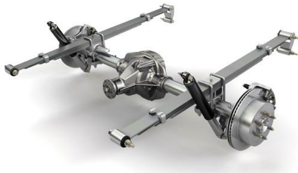
Figure 13 – Live axle with leaf springs. [27]
