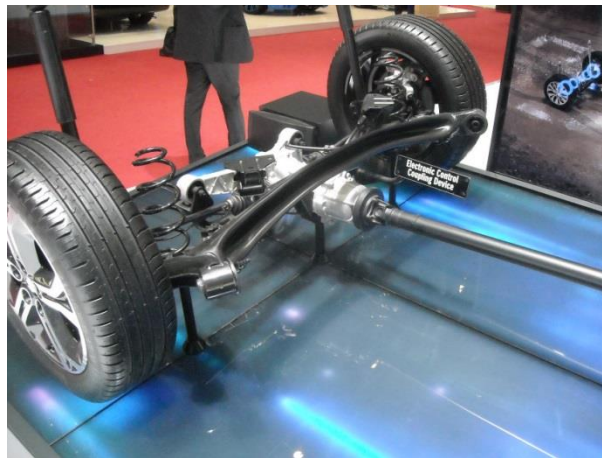
Figure 16 - Suzuki Vitara - driven rear torsion beam suspension. [31]
