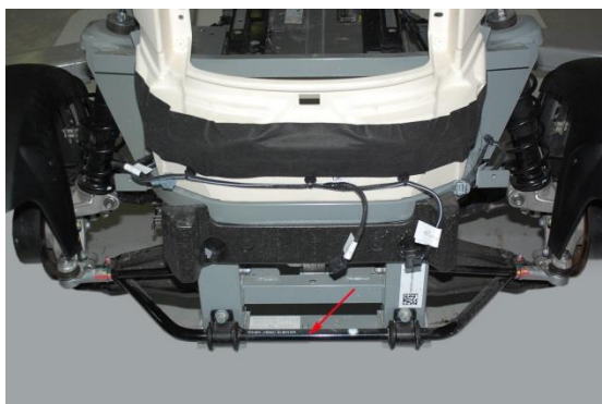
Figure 4 – Rear antiroll bar (stabilizer) of Twizy. [18]
