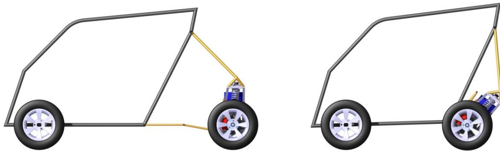
Figure 96 – Render of the folding mechanism, park mode length is 2110mm, ride mode length is 2810 mm.
