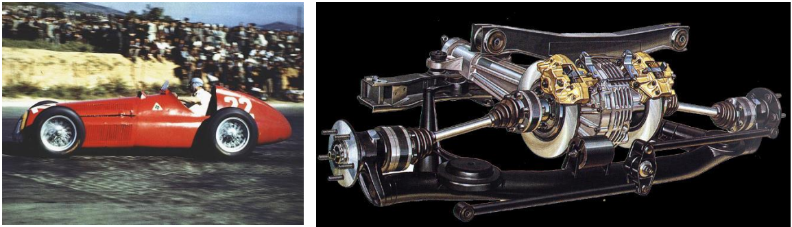
Figure 12 – left: Alfa Romeo 159 (1950) [26], right: Alfa Romeo De-Dion rear suspension from the '80s. [28]
