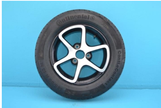
Figure 78 – The rear wheel of Twizy, wearing Continental Conti.eContact 145/80 R 13 75 M [18]
