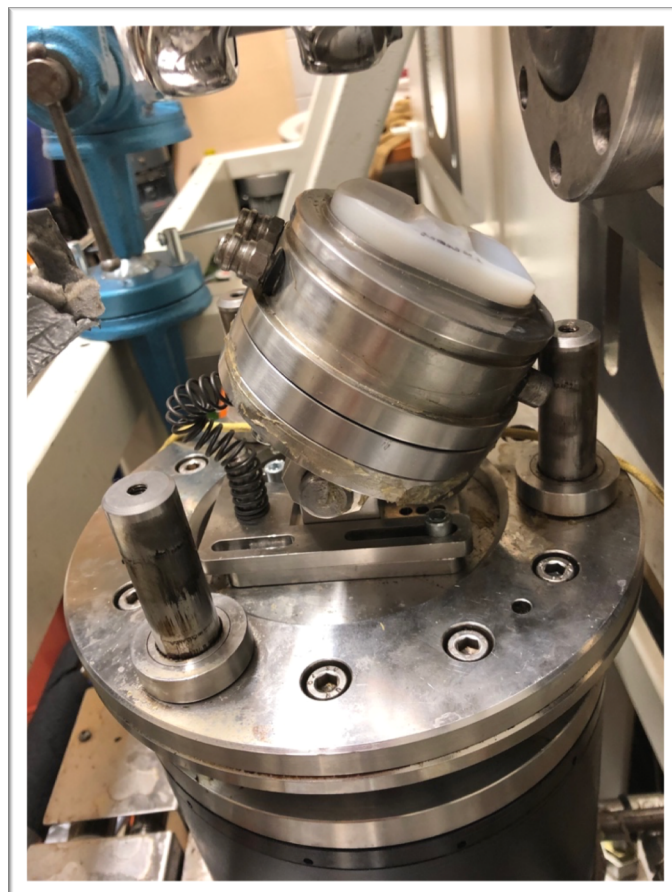
Figure 30: The position of the spring in the simulator
