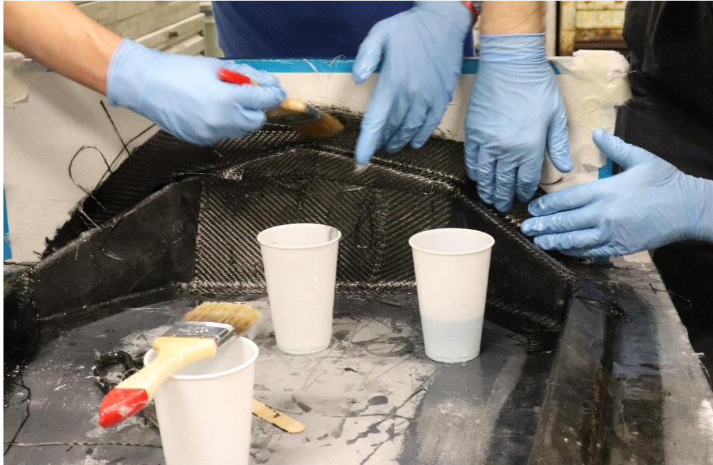
Obr 3. Laminace forem na monocoque FSE.08
