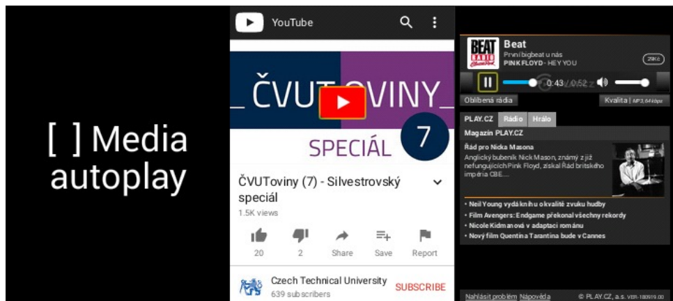
Figure 4.6: Examples of UI screens related to the media playing shows that even the medial content can be accessed quite easily: a) Media autoplay settings option, if selected audio and video content present in pages starts automatically, b) Playing video at youtube.com manually without autoplay option on using 'Play' button c) Playing internet radio.
