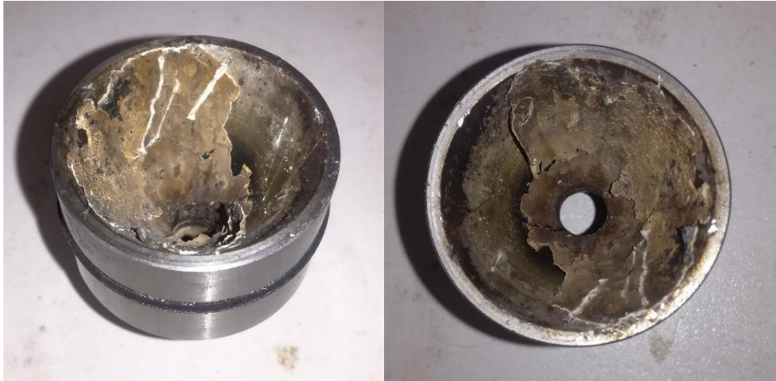
Fig. 30 – Convergent section of the nozzle covered with thin layer of ash
