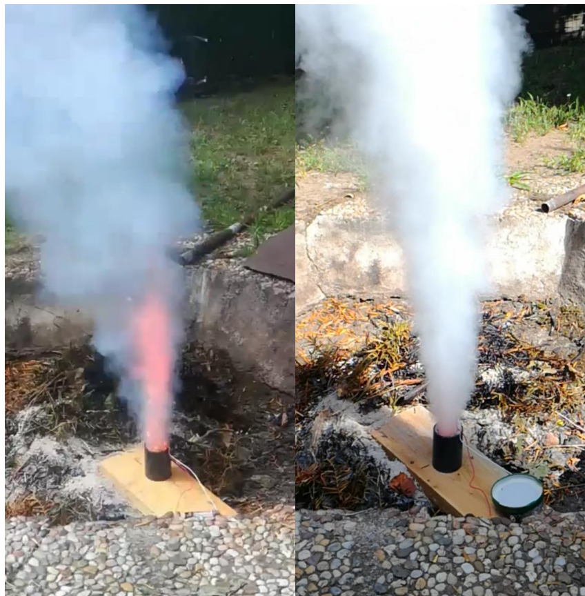
Fig. 14 – Comparison of two propellant grains with different manufacturing process. Compressed mixture on the left, casted mixture on the right.
