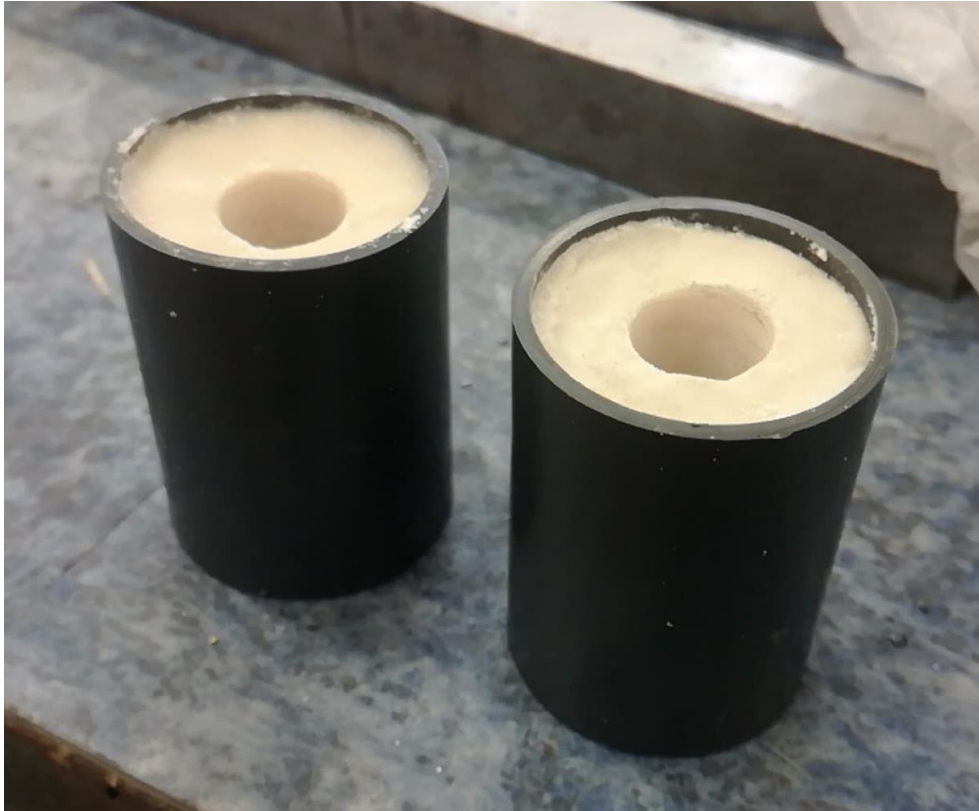
Fig. 16 – Finished BATES propellant grains.
