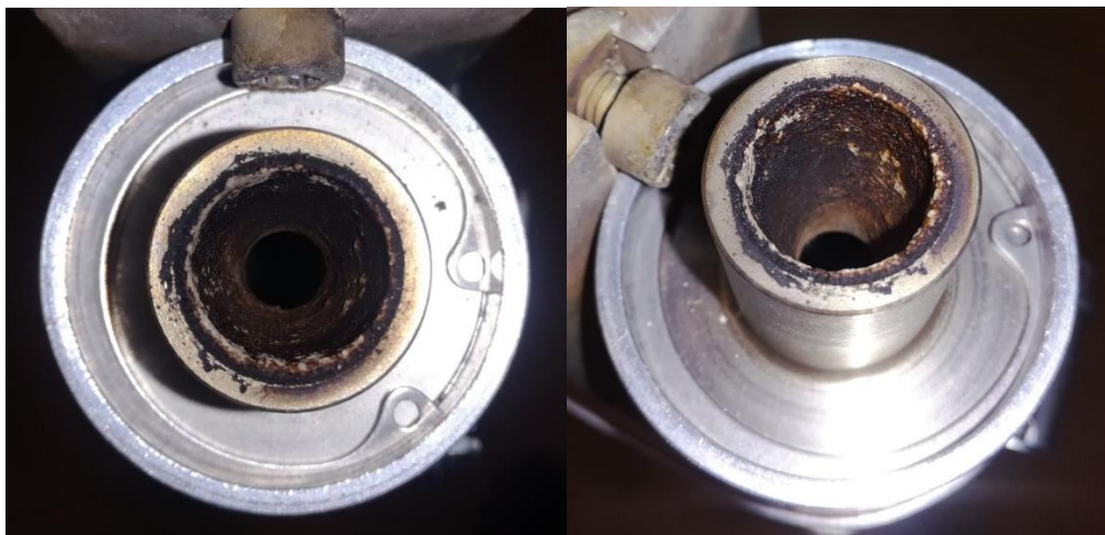
Fig. 26 – Immediate condition of the nozzle directly after the test
