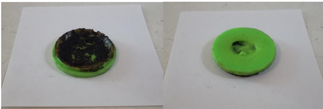
Fig. 35 – Combustion chamber stopper
