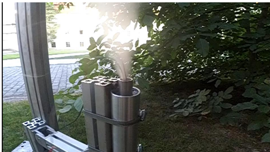
Fig. 23 – T+1,95s (wires fly out of the nozzle as the thrust abruptly increases)
