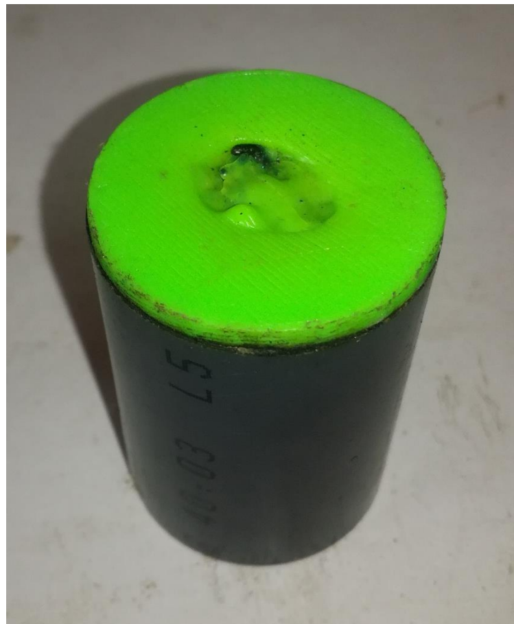
Fig. 29 – The damaged plastic stopper still connected to the PVC inhibitor
