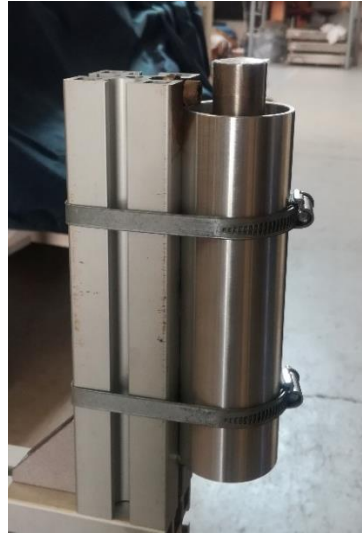
Fig. 19 – Experimental rocket motor mounted to the measuring apparatus
