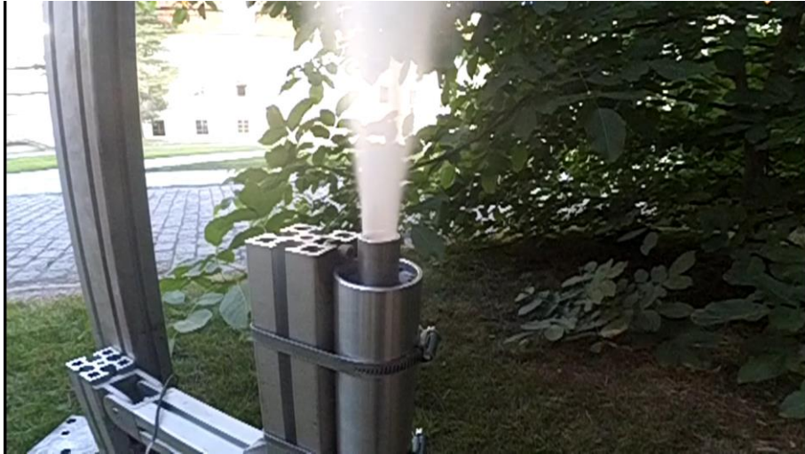
Fig. 24 – T+2,7s – the peak thrust with possible glimpse of Mach diamond effect
