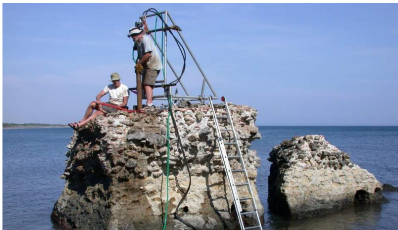
Figure 6. Portus Cosanus , ROMACONS coring process at a hydraulic concrete pila . (Brandon et al., 2014)
