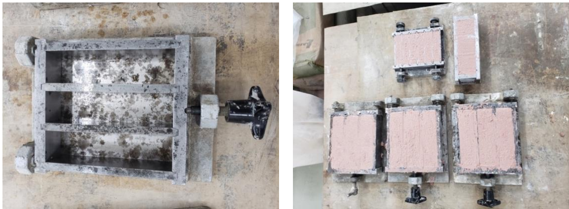
Figure 15. (left) Empty three-gang mold; (right) mortar-filled molds for Mix 1.
