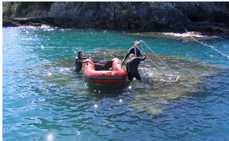
Figure 1. Typical pila being cored for experimental trials during the ROMACONS project. (J. Oleson et al., 2004)
