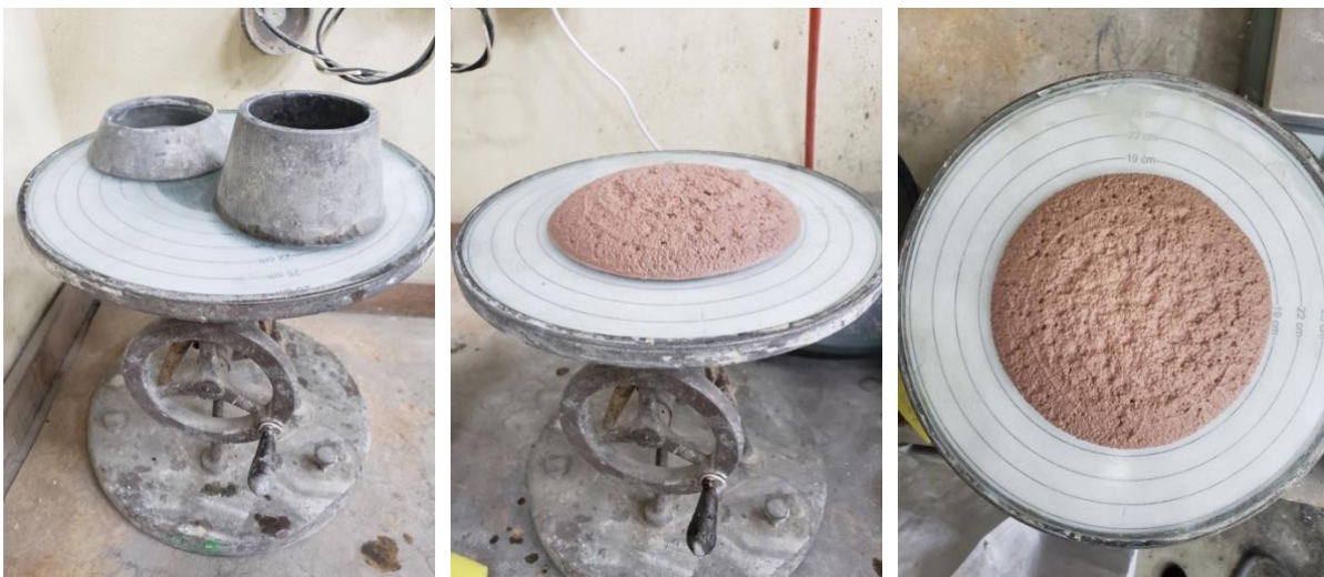
Figure 14. (left) Flow table setup with empty mold; (middle &amp; right) spread mortar after completion.
