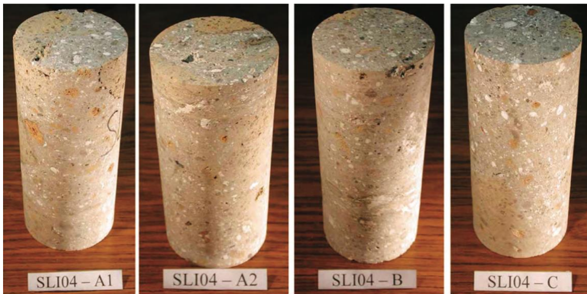
Figure 7. Four sub-core specimens shaped from a ROMACONS full-length core with a typical diameter of 86.5 mm and a length of 175 mm. (Brandon et al., 2014; J. Oleson et al., 2004)
