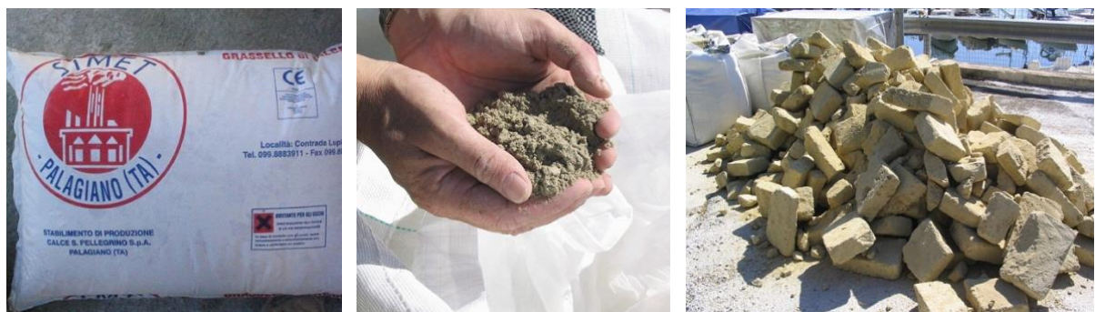
Figure 9. Raw materials for the reproduction of the Brindisi pila ; (left) lime putty; (middle) pozzolana; (right) tuff aggregate. (J. P. Oleson et al., 2006)
