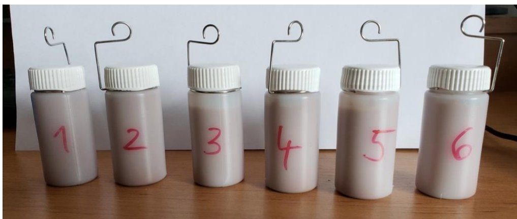
Figure 16. Six 20ml paste specimens immediately before entering the isothermal calorimeter.
