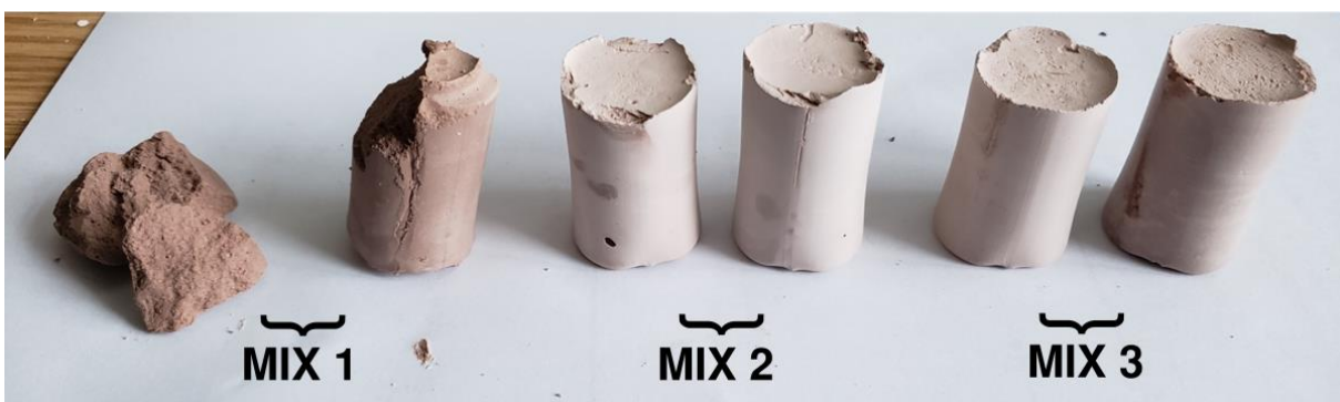
Figure 22. All three paste mixes after being cut out of their plastic vials 14 days after being mixed.
