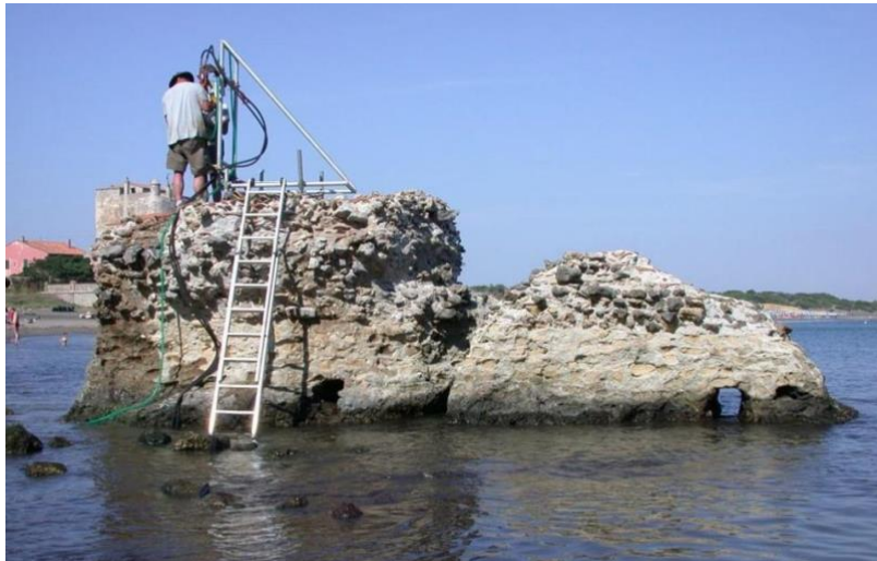
Figure 5. Portus Cosanus , ROMACONS coring process at a hydraulic concrete pila . (Brandon et al., 2014)
