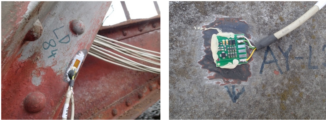
Figures 40 and 41. Monitoring Equipment: Strain Gauge (left); Accelerometer (right) (Ryjáček, 2019).
