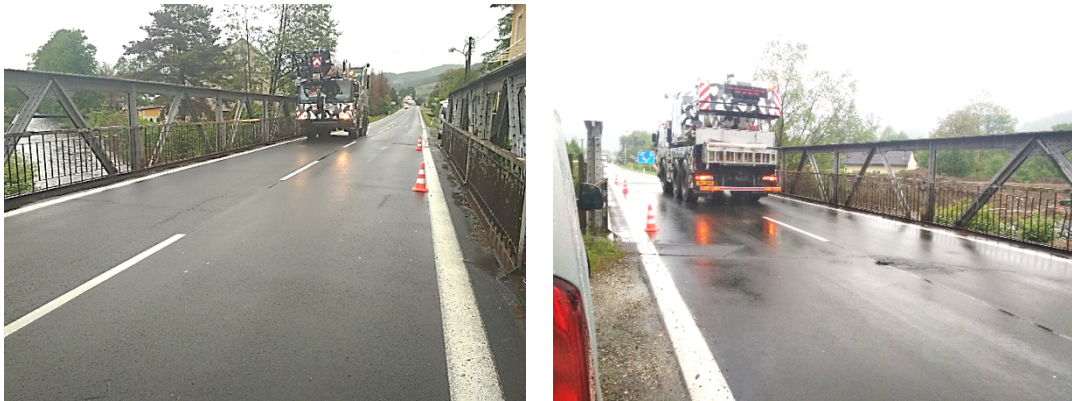
Figures 43 and 44. Load Test Being Performed: In the Lane (left); On the Axis (right) (Ryjáček, 2019).
