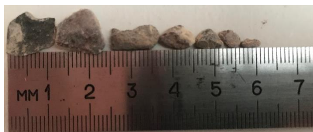
Figure 24 - Typical Aggregate Sizes within Mortar.
