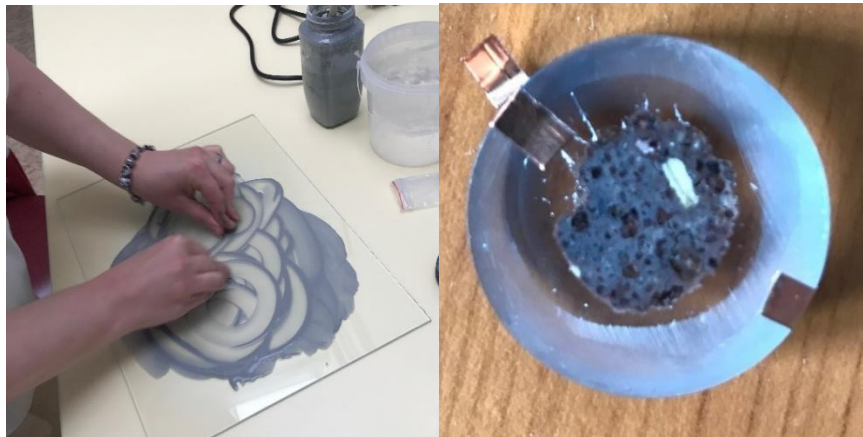
Figure 21 - Silica Oxide Polishing of Sample (Left). Prepared Sample (Right).
