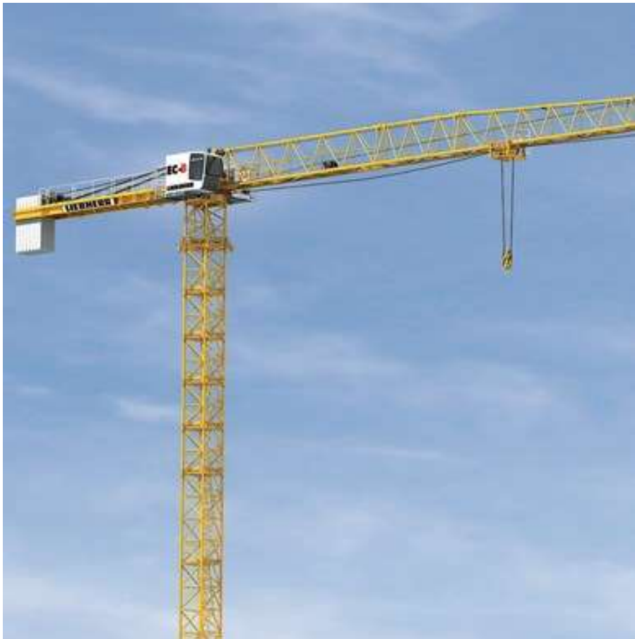
Obr. 13 Jeřáb typu Flat-Top Liebherr 172 EC-B 8 Litronic [17]
