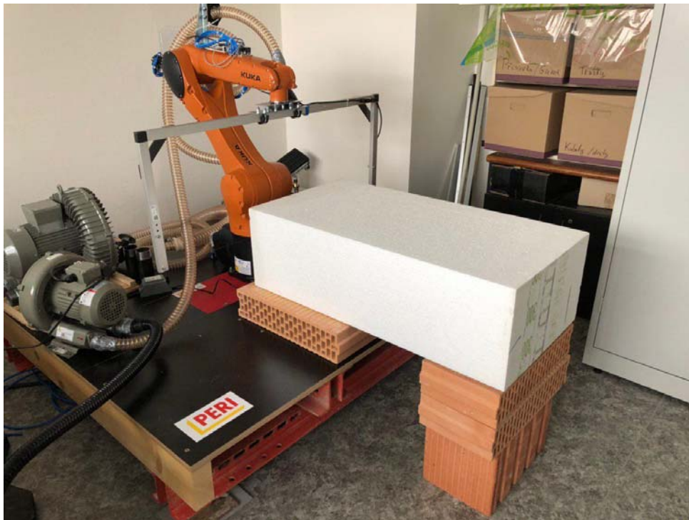
Fig.50 KUKA robot with hot-wire tool. Source: author
