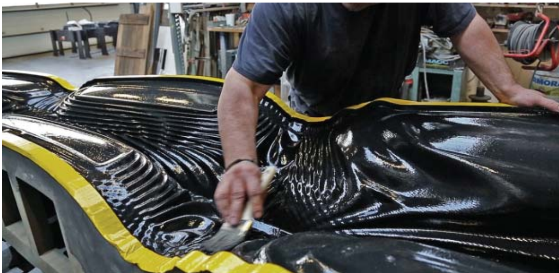
Fig.26 Application of the release agent. Source: [8]
