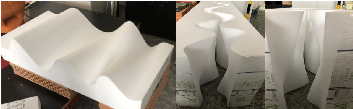
Fig.52 The EPS formwork. Source: author
