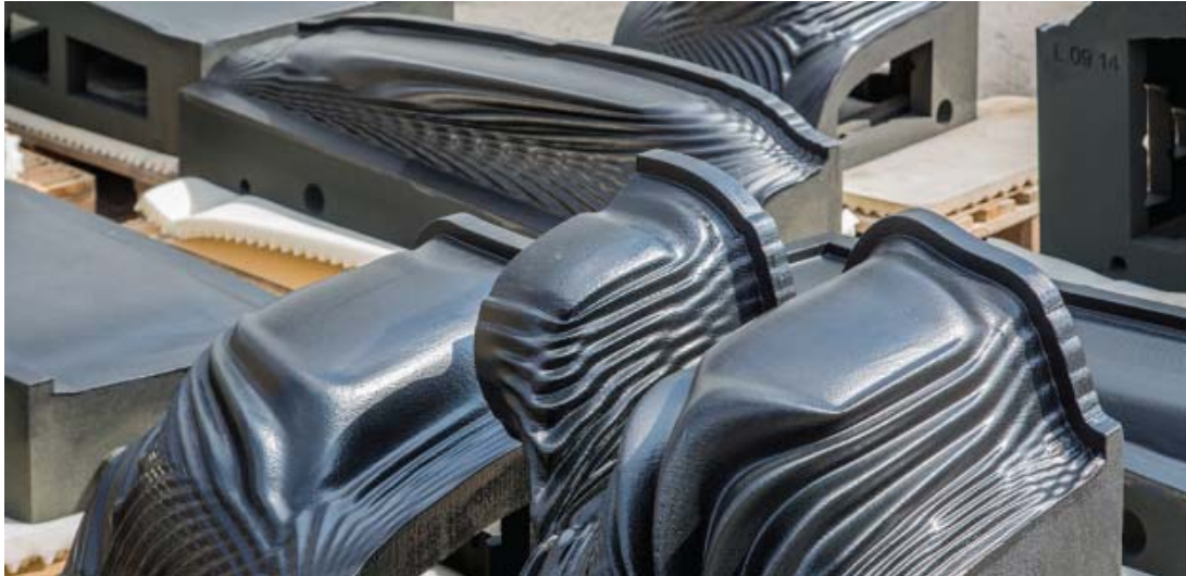
Fig.27 3D printed parts coated with polyester resin.
