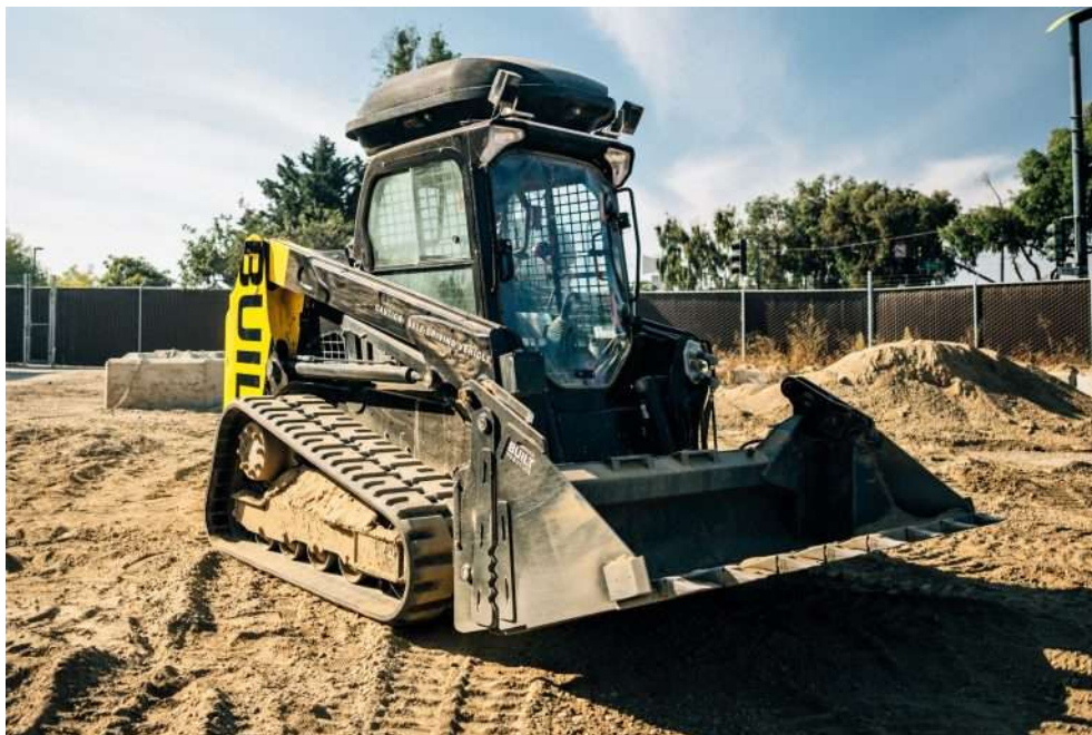
Fig. 30 Autonomous Track Loader from The Built Robotics. 122
