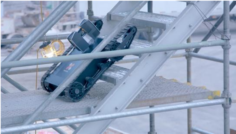
Fig. 31 Doxel inspection robot. 124
