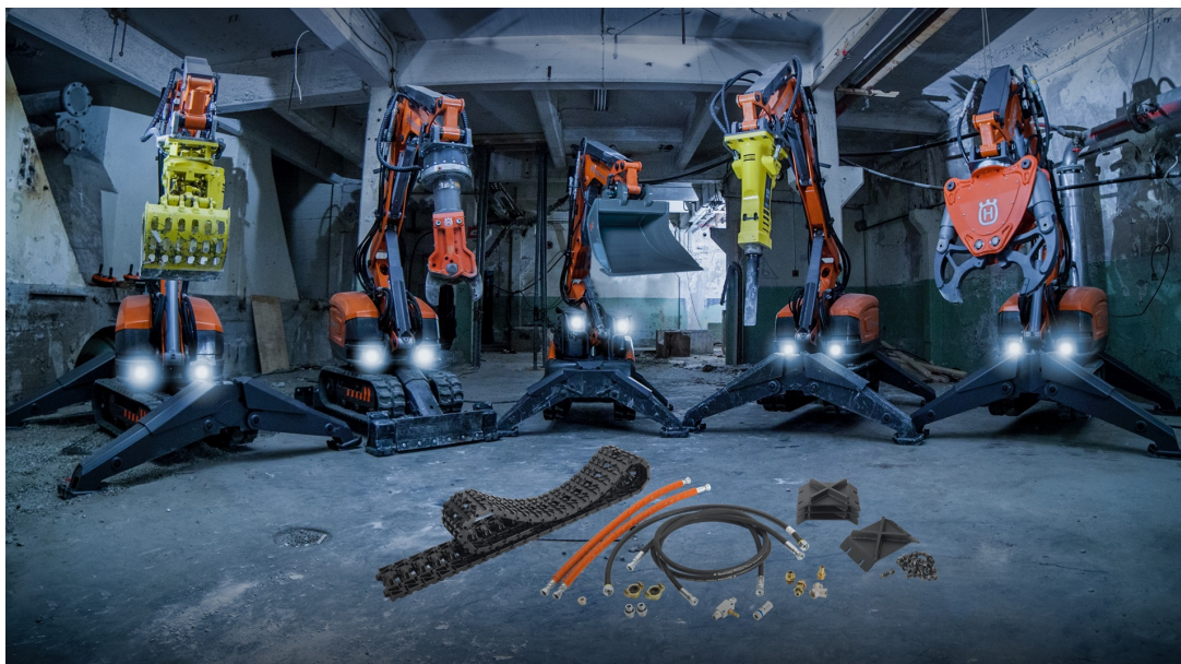
Fig. 20 Multi-tooled demolition robot by Husqvarna. 100
