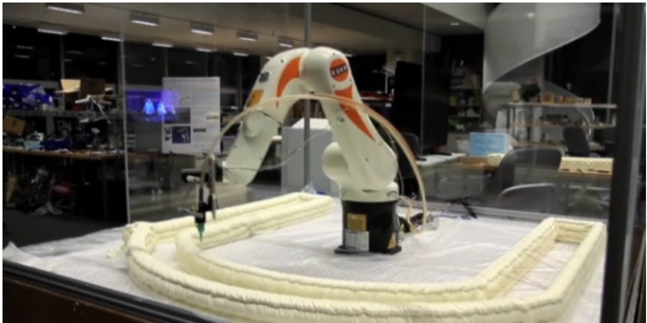
Fig. 37 An example of 3D printing robotic arm. 138
