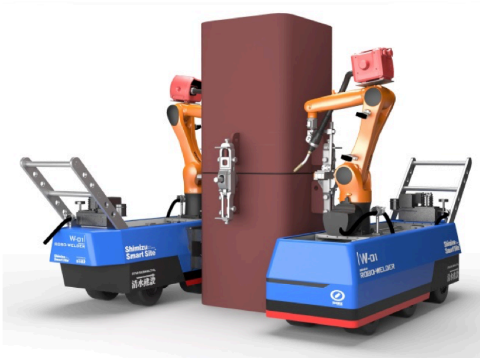
Fig. 22 Welding robot from Shimizu corporation. 105
