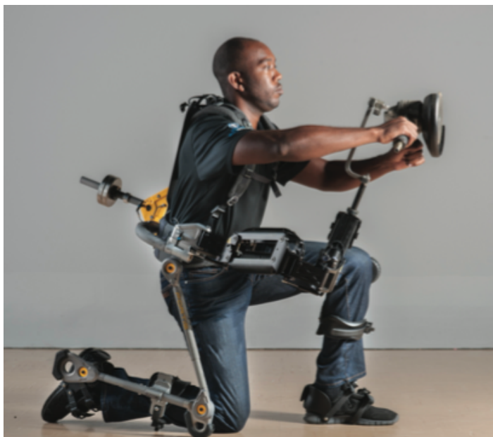
Fig. 29 FORTIS exoskeleton demonstration. 118 [85 p. 207]
