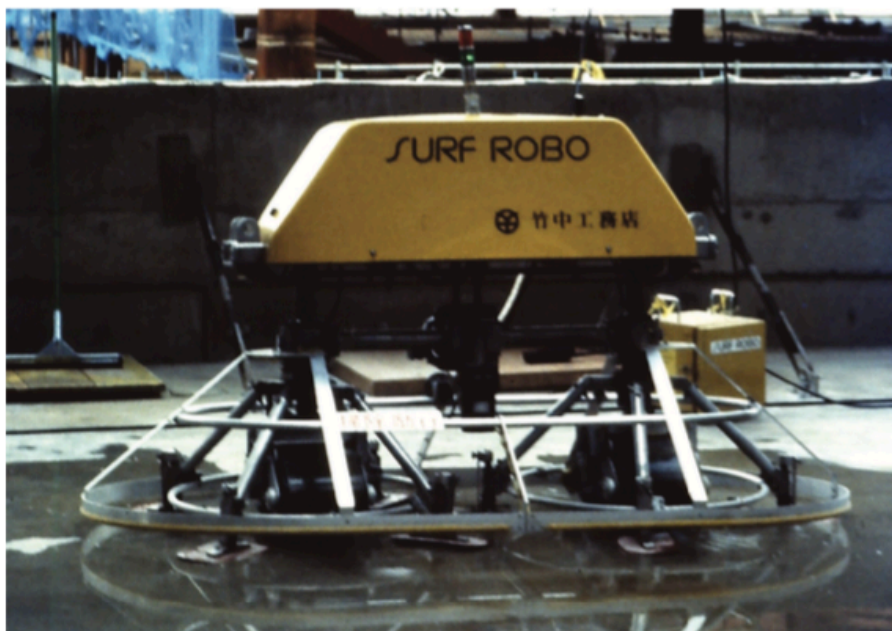
Fig. 42 Surf Robo concrete finishing robot. 150
