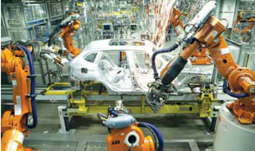
Fig. 11 Robotic arm welding a car frame. 63
