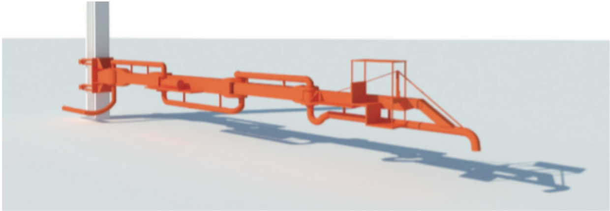
Fig. 40 Scheme of a concrete laying robot. 146
