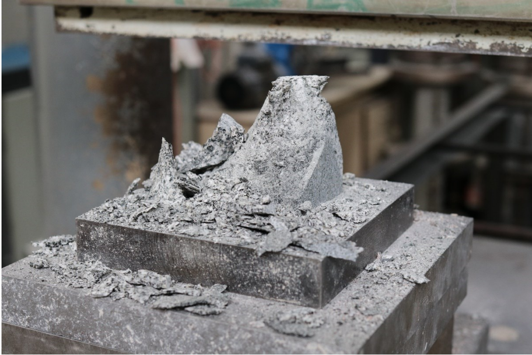
Fig. 16 Destroyed sample after UCS test (picture: M. Jonáš)
