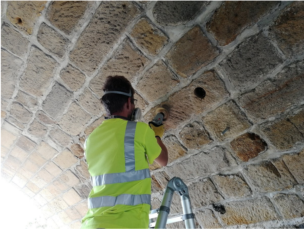
Fig. 14 Surface grinding for humidity metering and Schmidt hammer measurement (picture: J. Zatloukal)
