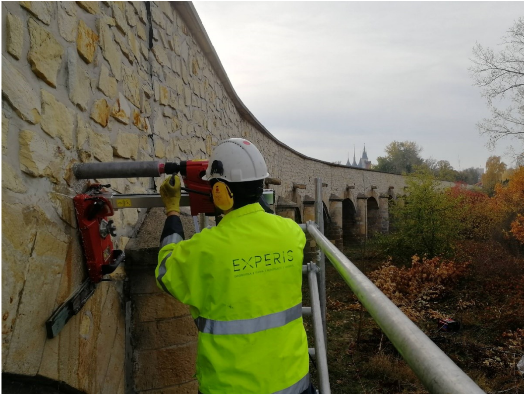
Fig. 9 Extraction of sample using diamond core drilling at bridge near Louny (picture: M. Jonáš)
