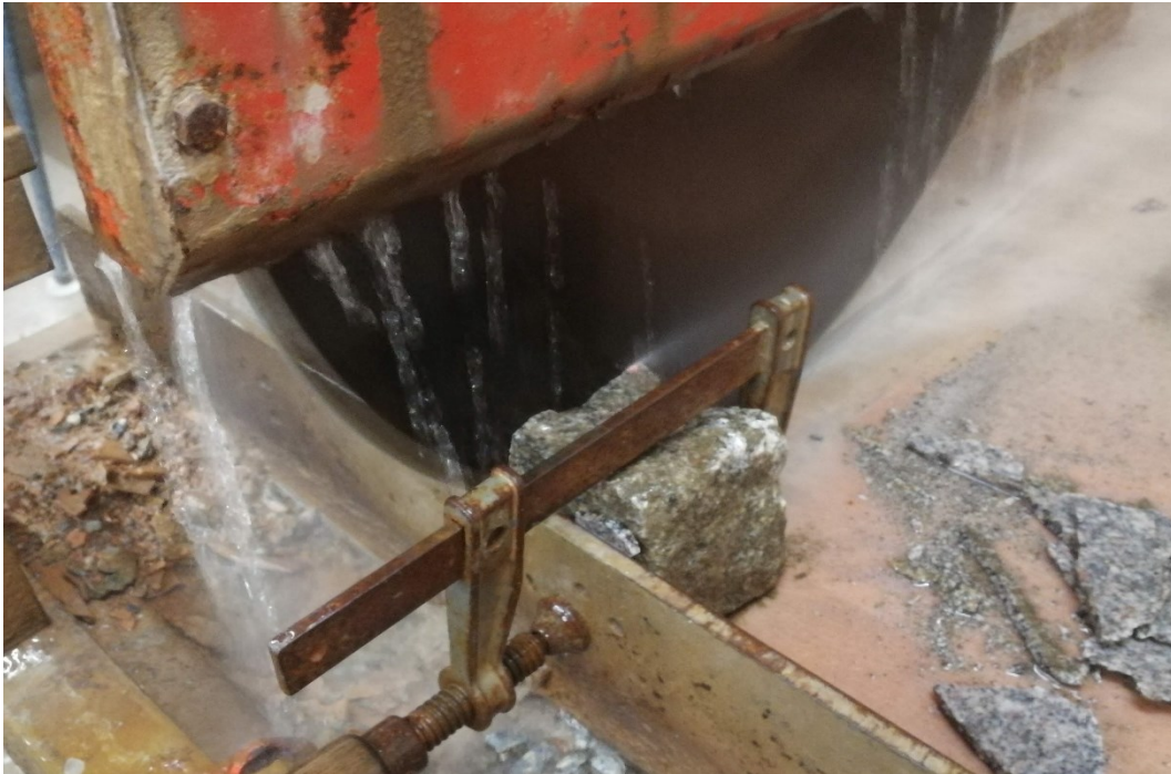
Fig. 10 Diamond saw cutting paving sett (picture: M. Jonáš)
