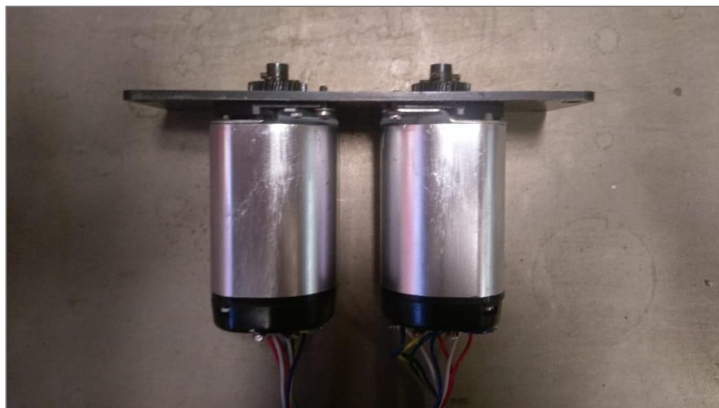
Figure 7: Existing Stepper Motors
