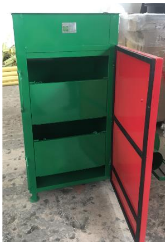
Figure 20. 93.75 kg Vertical coffee dryer.
