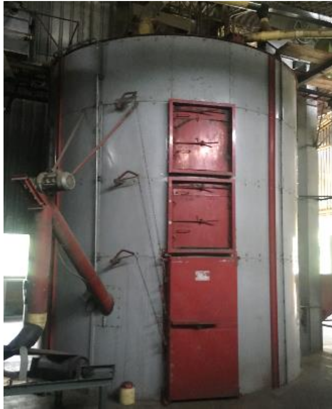
Figure 15. Dryer with mechanical agitation of the coffee in the chambers and discharge with screw.
