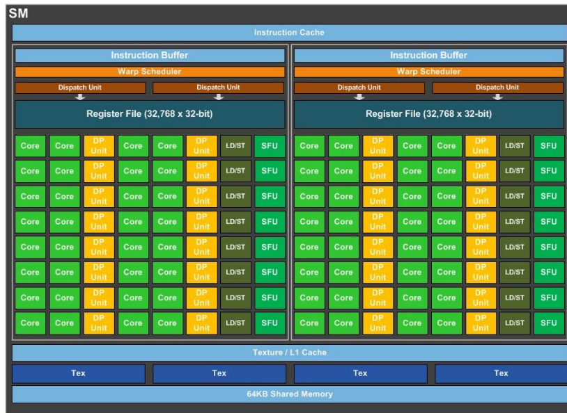
Figure 2.7: GP100 Pascal micro-architecture [9]
