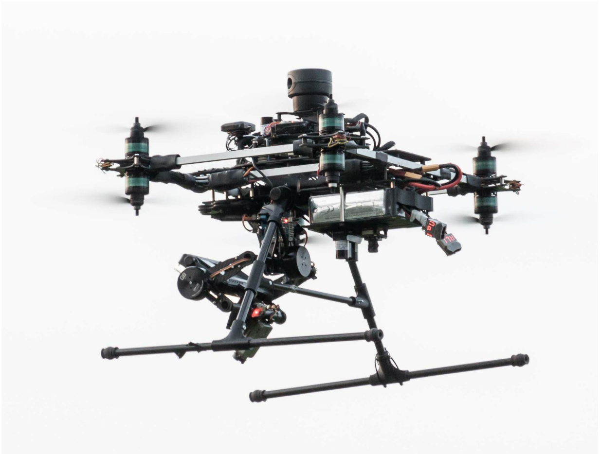
Figure 6.13: Specialized platform developed within Multi-robot Systems group for scanning of historical buildings interiors during its deployment in the experiment presented in Section 6.3.
