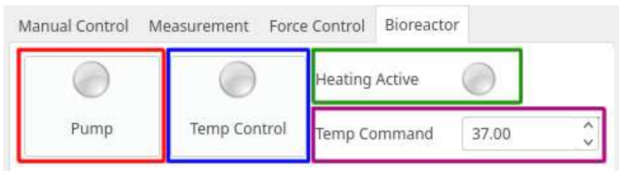
Figure 4.30: Temperature control plugin of the user interface
