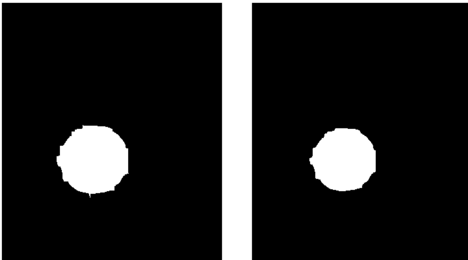
(a) : Result of closing operation until one shape remaining
