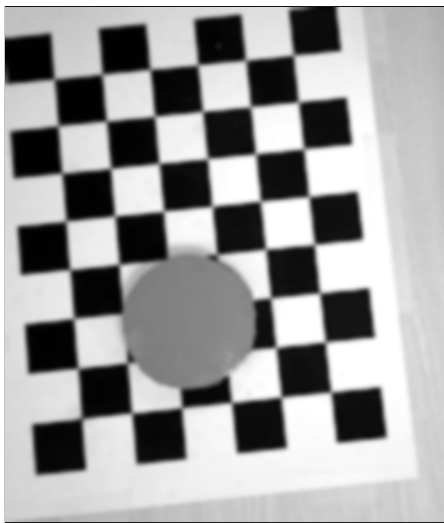
(a) : Gaussian blur applied to grayscale version of RGB image
