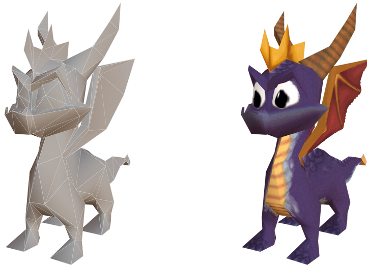
Figure 2.1: The main character from Spyro the Dragon, game released in 1998. On the left is mesh geometry with a wireframe of about 400 triangles. On the right, a mesh with textures. (Image courtesy of Activision Publishing, Inc. Game developed by Insomniac Games, Inc.)
