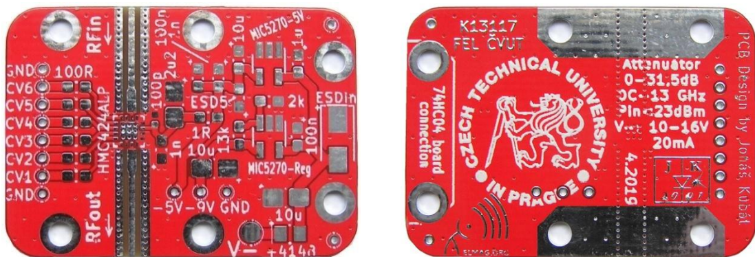
Obr.43 - DPS zeslabovače HMC424A z JLC PCB (FR4, HASL)
