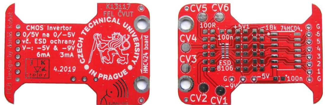
Obr.44 - DPS invertoru 74HC04 z JLC PCB (FR4, HASL)
