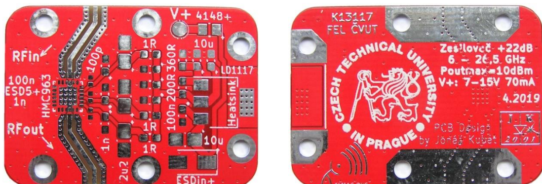
Obr.32 - DPS zesilovače HMC963 z JLC PCB (FR4, HASL)
