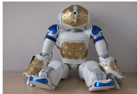
(b) : Artificial skin mounted on NAO robot
