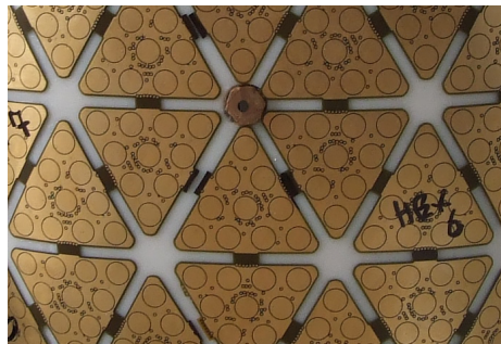
(a) : Physical artificial skin sensors
