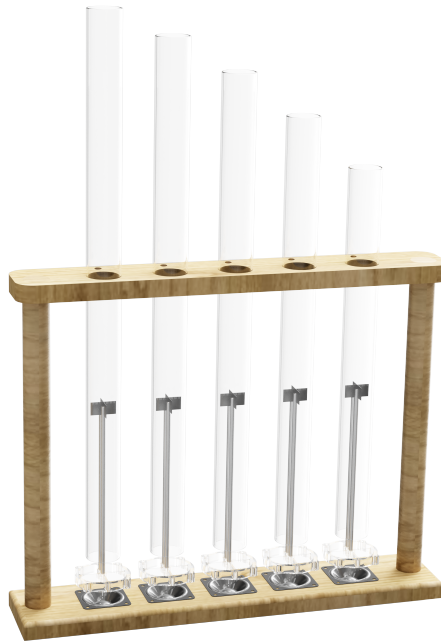
Figure 6.1: Original in-line design concept of Rijke tube organ.
