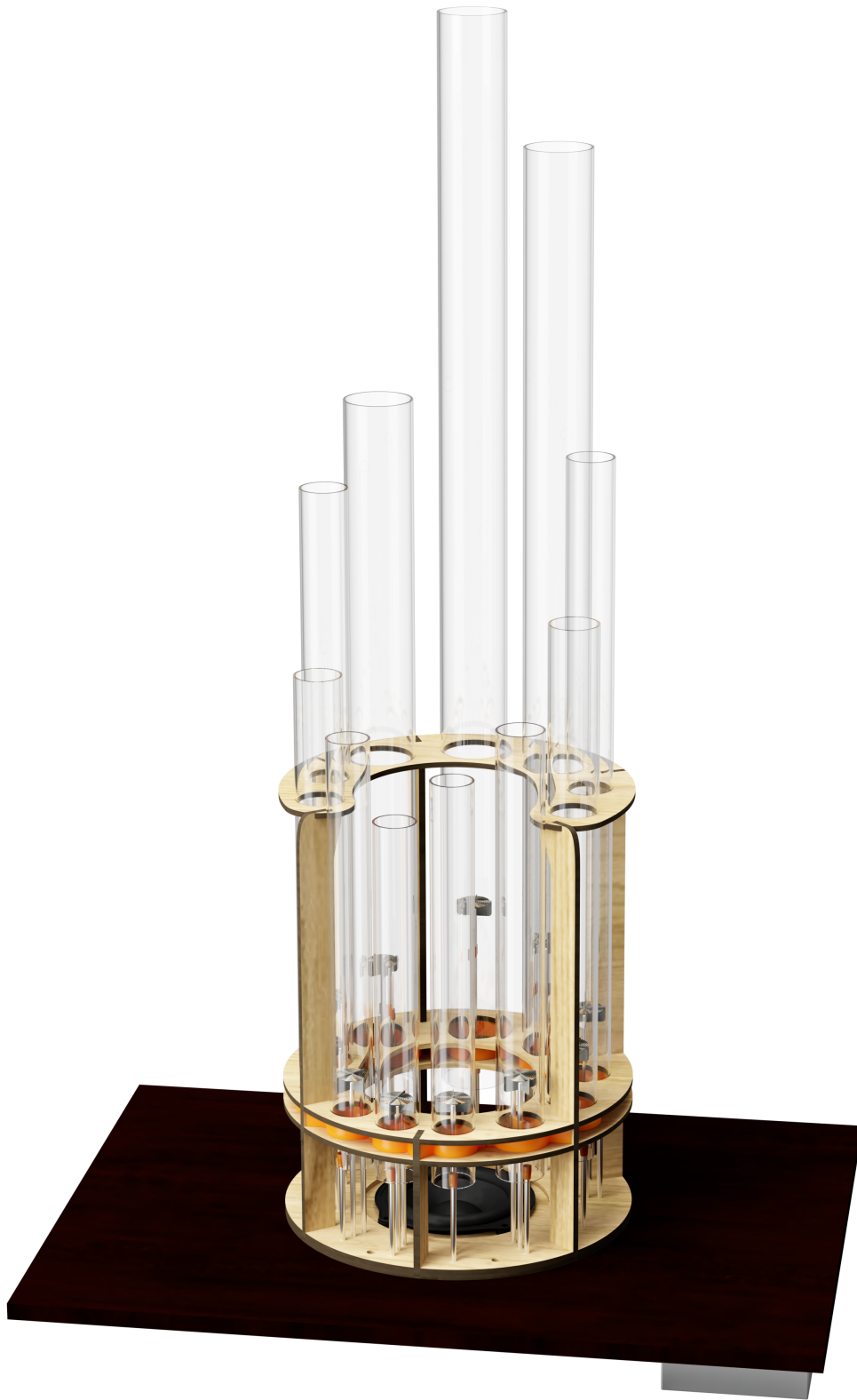
Figure 6.8: 3D model rendering of the designed Rijke organ.
