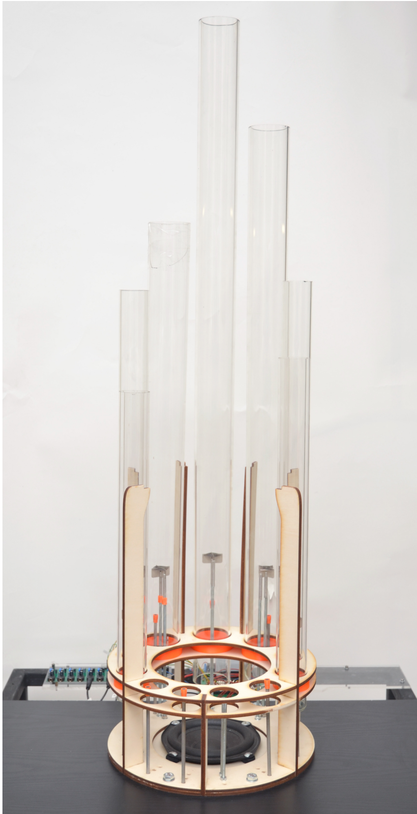
Figure 6.9: Photograph of the Rijke organ build.
