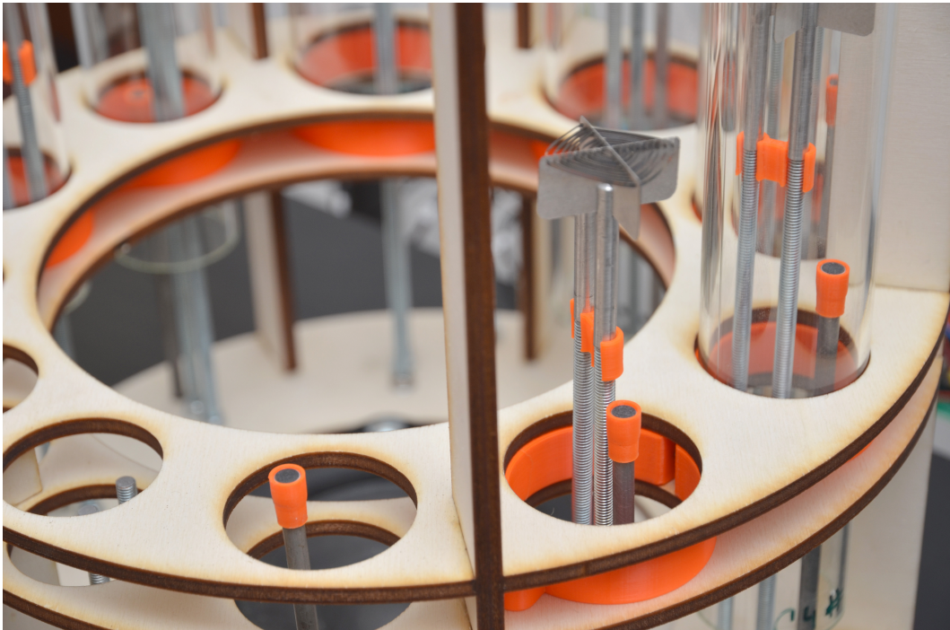
Figure 6.4: Final designed microphone sensors installed in the organ.
