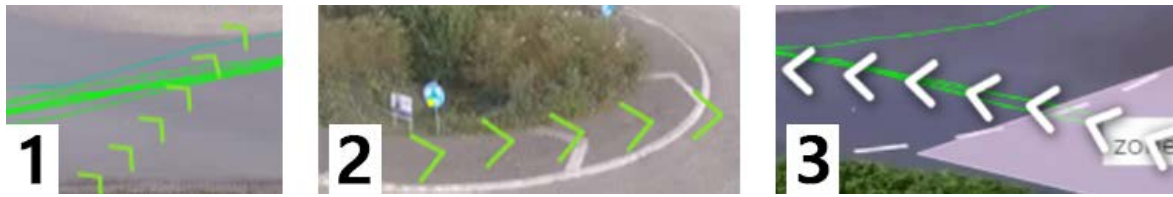
Figure 4.1: Evolution of direction arrows. Thanks to its size, color and black shadow, the third option is visible on the majority of backgrounds.
