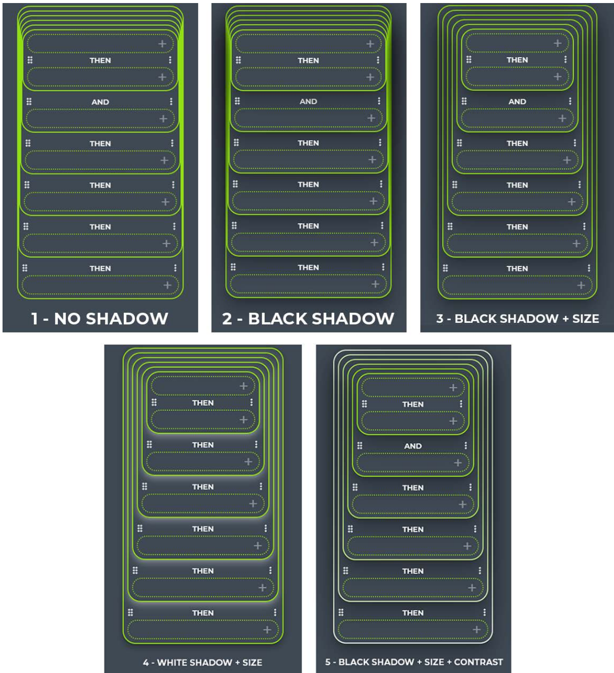
Figure 3.12: Evolution of the high-fidelity prototype for the binary tree structure of the composite filter expression where number 1 represents the initial state that is not well readable, and the best design - number 5 implementing three factors for a better depth recognition.
