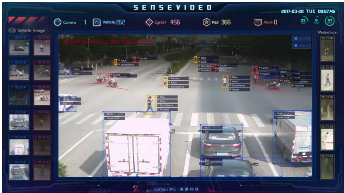
Figure 2.5: Application by SenseTime showing real-time object detection together with its detected attributes.
