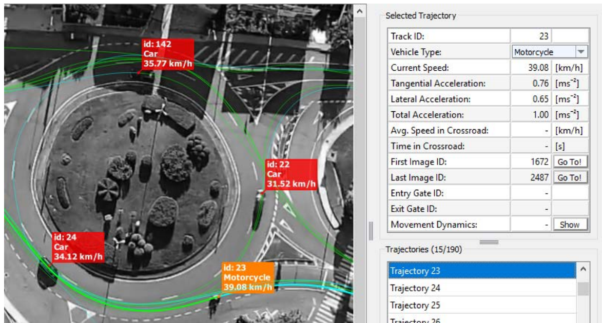
Figure 2.4: Application by DataFromSky showing detected objects within a video together with detailed information.
