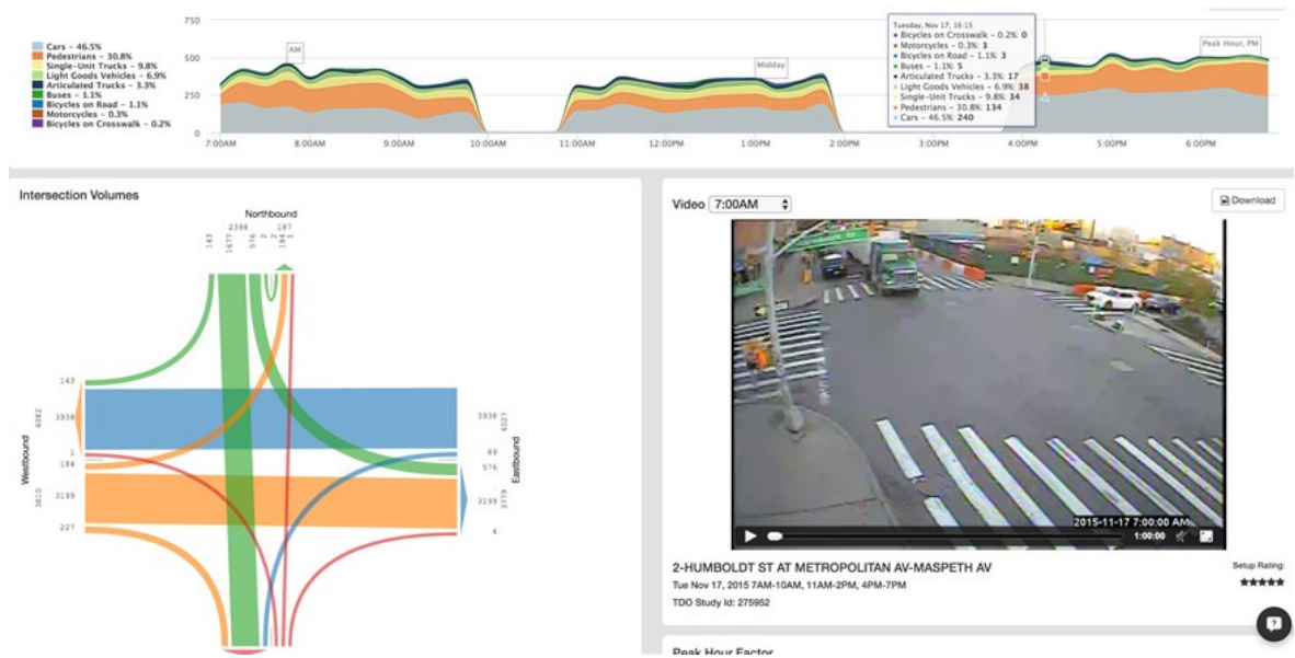
Figure 2.3: DataLink by Miovision showing intersection volumes on the left and camera preview on the right
