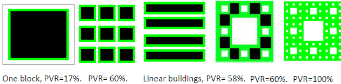
Figure 15 Passive Volume Ratios (PVR) for different perimeter blocks (Salat and Bourdic, 2012)
