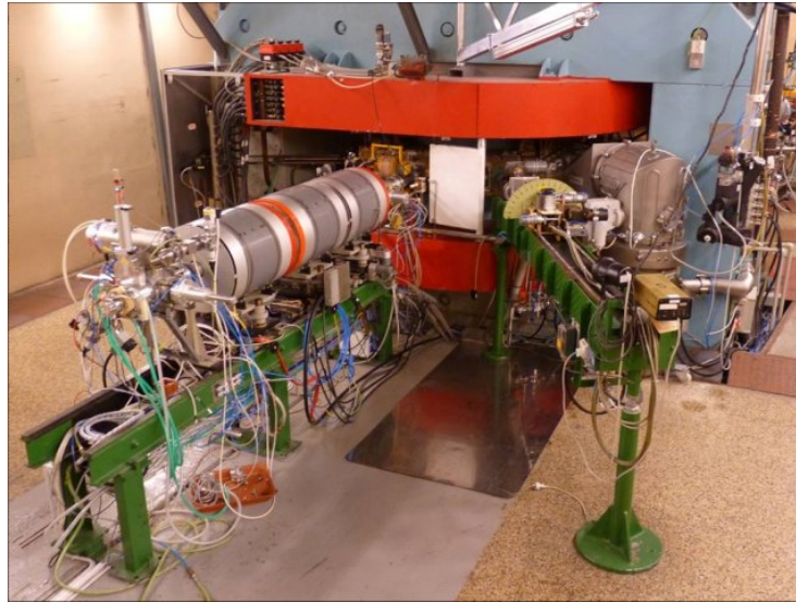
Figure 2.7: A photo of the cyclotron U-120M at NPI, Řež. The main magnet core is visible in blue and its two pole windings are visible in red with a vacuum chamber in between. The vacuum chamber itself is not visible well, as the view is obstructed by a cyclotron technology and beam instrumentation equipment. An extraction beam pipe is visible on the left green support with several correction magnet mounted. (Source: [23])
