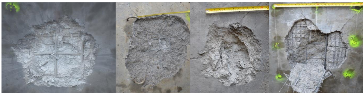
Figure 7. Specimen No.17 after contact blast loading, 2.8 kg charge left left contact side, left right soffit, 4.2 kg charge right left contact side, right right soffit
