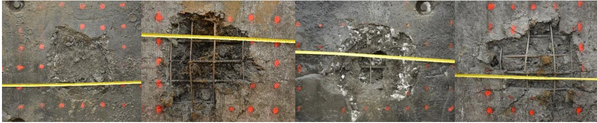
Figure 12. Specimen No. 23 after contact blast loading, 2.8 kg charge left left contact side, left right soffit, 4.2 kg charge right left contact side, right right soffit
