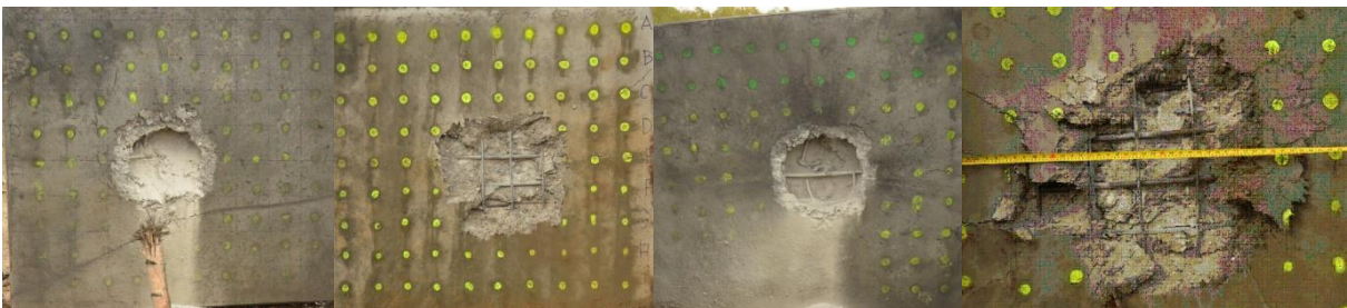
Figure 9. Specimen No. 19 after contact blast loading, 2.8 kg charge left left contact side, left right soffit, 4.2 kg charge right left contact side, right right soffit
