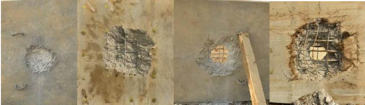
Figure 4. Specimen No. 14 after contact blast loading, 1.4 kg charge left left contact side, left right soffit, 2.8 kg charge right left contact side, right right soffit
