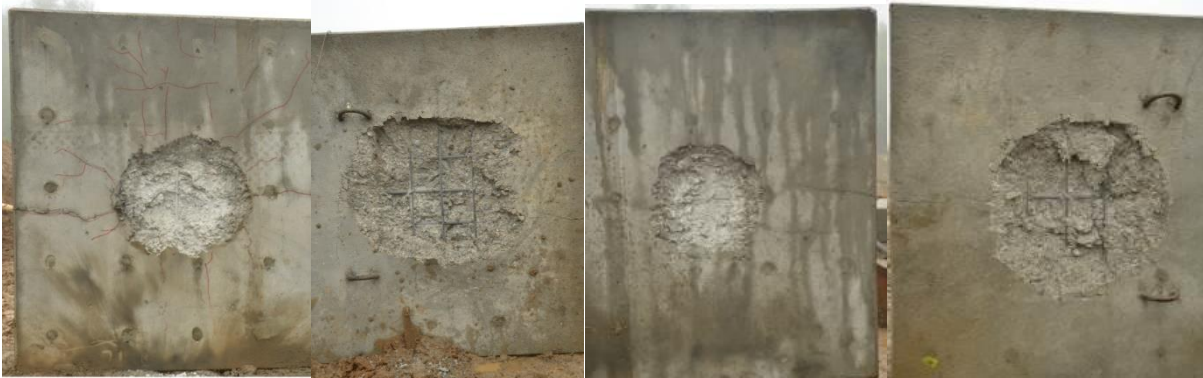
Figure 2. Specimen No. 12 after contact blast loading, 1.4 kg charge left left contact side, left right soffit, 1.0kg charge right left contact side, right right soffit
