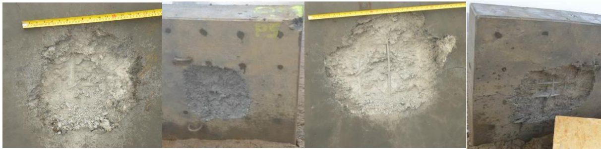
Figure 6. Specimen No. 16 after contact blast loading, 2.8 kg charge left left contact side, left right soffit, 2.0 kg charge right left contact side, right right soffit
