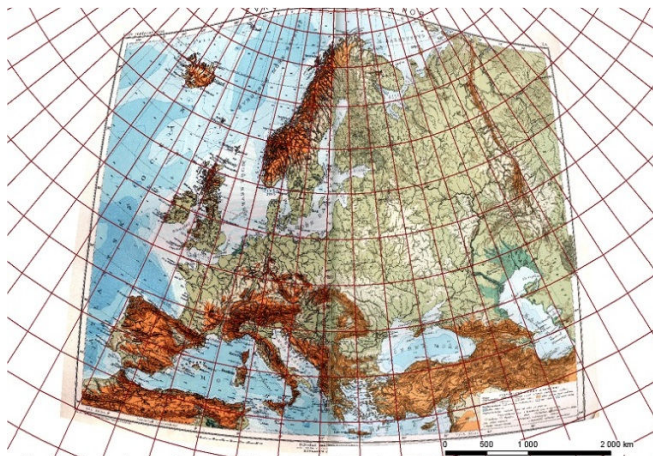
Fig. 11 Plate Carrée (second order polynomial transformation) to Albers projection
