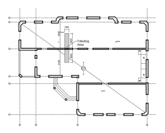
2.3.2- Estimation 1 m self-weight of the inner wall
