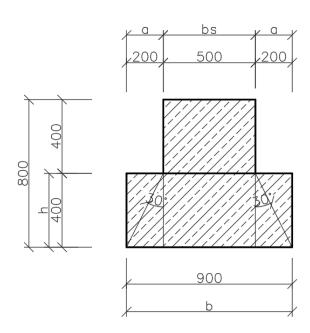
Design of Strip Footing is 0.9 m width and 0.4 m depth.
