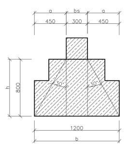
Design of inside Strip Footing is 1.2 m width and 0.8 m depth.
