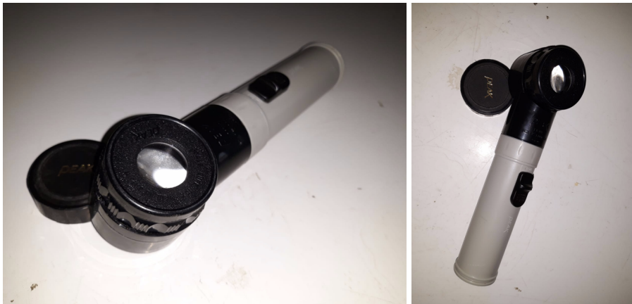
Obr. 47, 48: Lupa Peak 2028 Light Scale Loupe 10x
