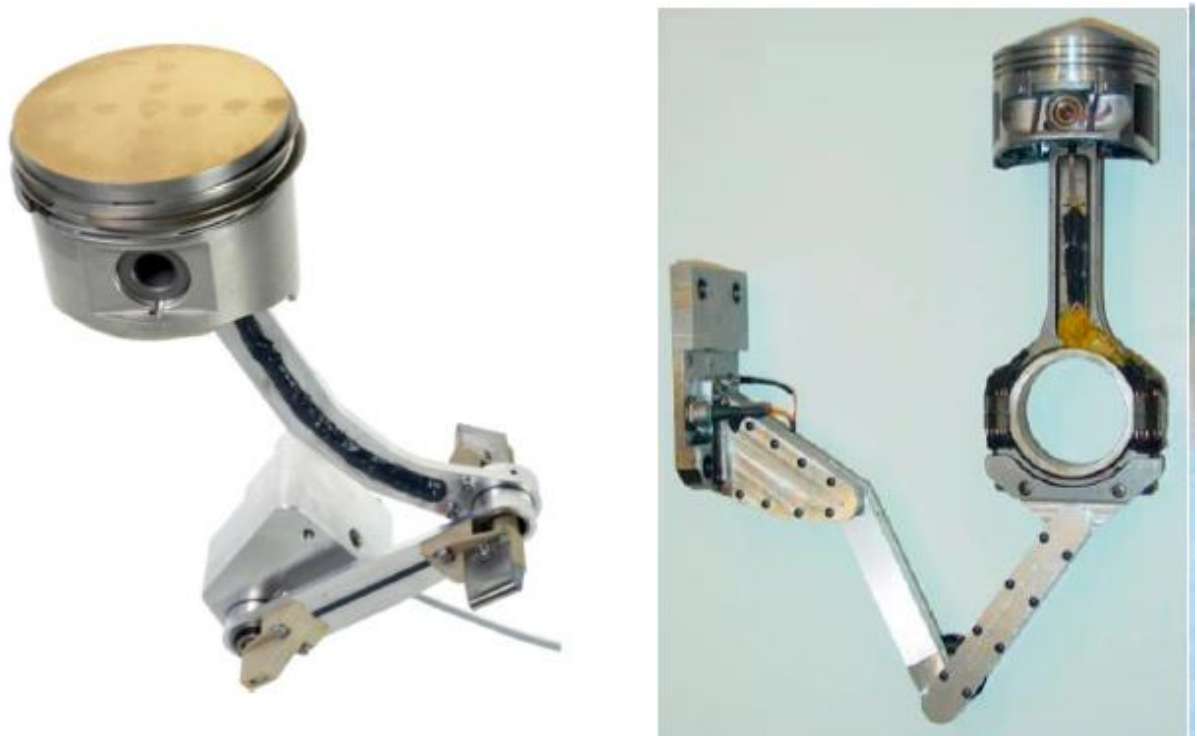
Figure 2.25: (Left) Grasshopper Linkage [17]; (Right) Mechanical Telemetry System [27]
