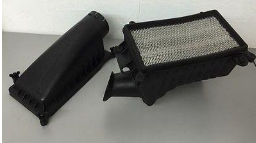
Figure 25. Air cleaning assembly.
