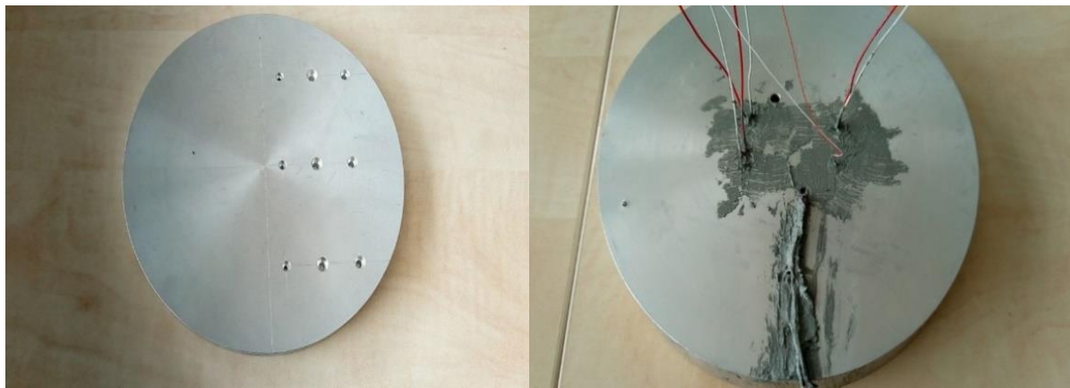
Figure 3-2: Trial installation of thermocouple wires
