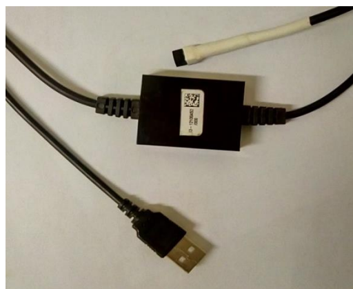
Figure 4-4: Telemetry Charging unit
