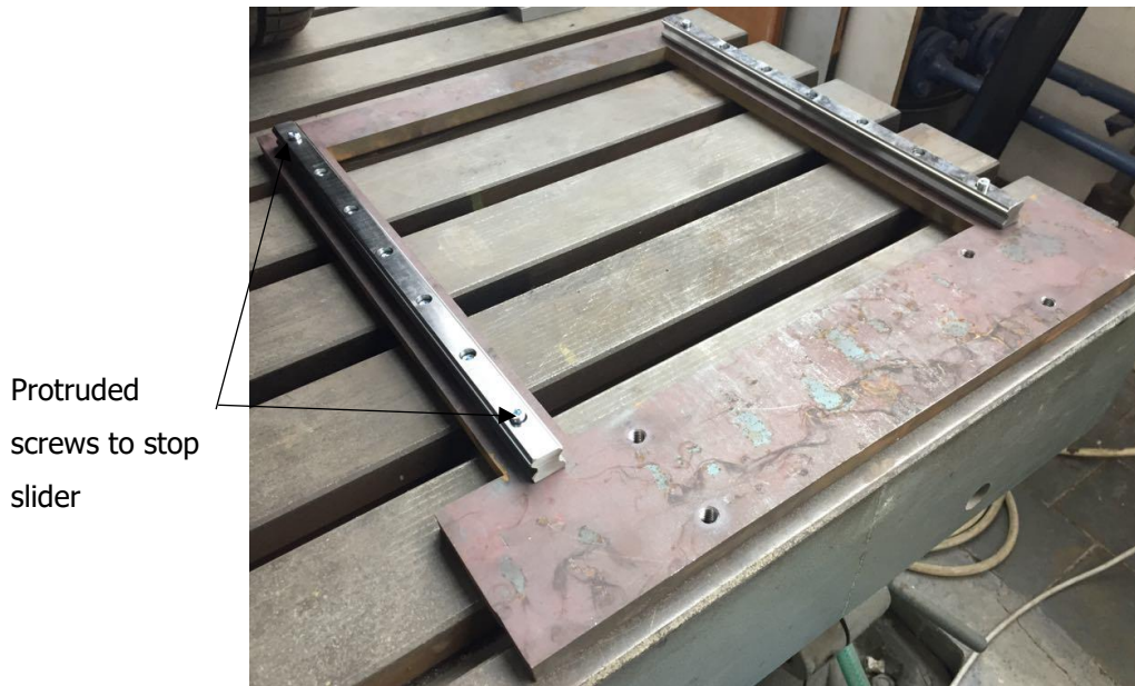
Figure 3-14: Fabricated slider base with installed rails
