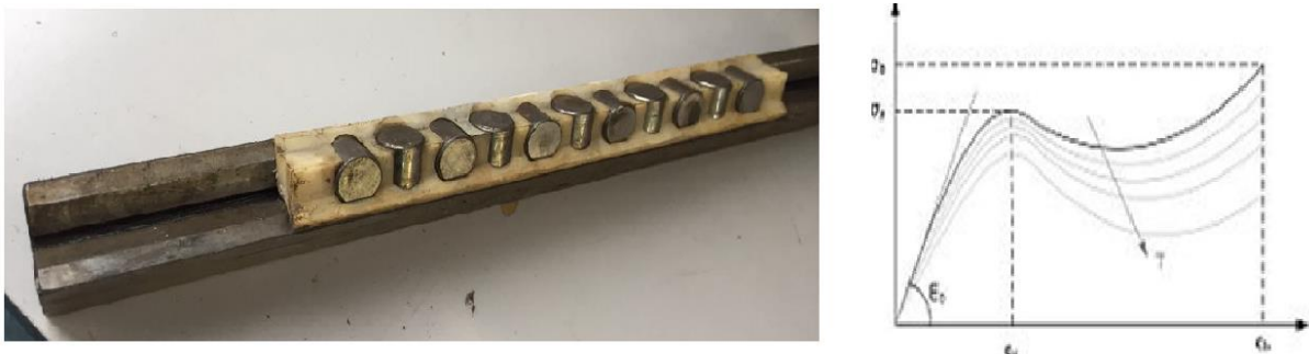
Figure 3-7: (a) soft plastic linear guides ; (b) Stress-strain graph of a thermoplastic POM [10]
