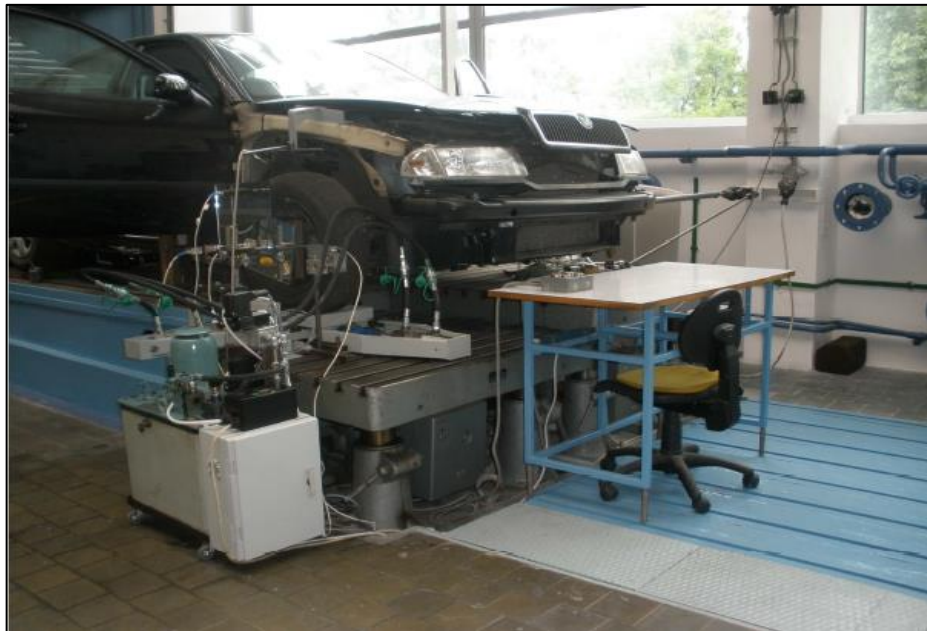
Figure 1-1 : Elastokinematics measurement test bench in CVUT Lab, Juliska (2011) [2]
