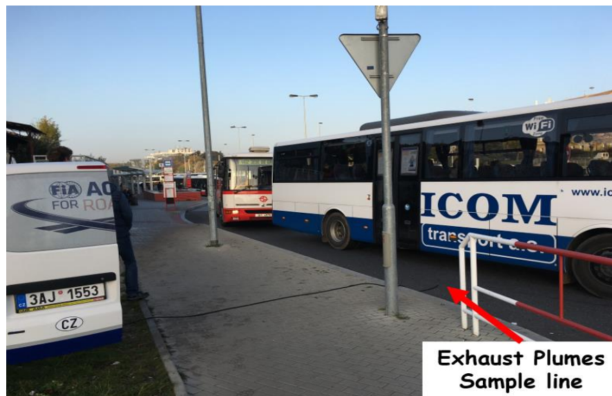
Figure 3.2 The van carrying the instruments was placed on the side of the road with an extending sample line
