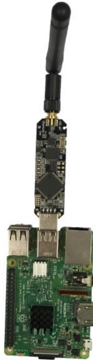
Figure 47.: Implementation of Ubertooth One
