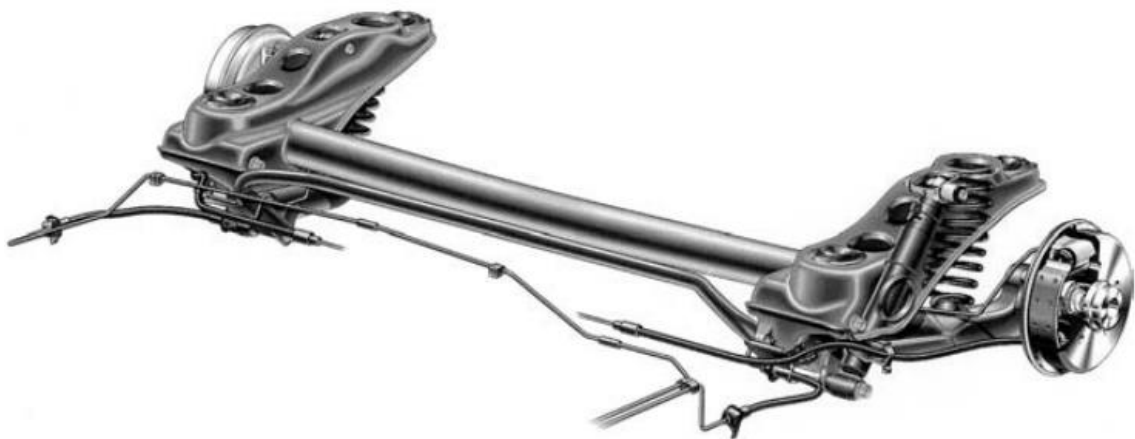
Figure 2.3: Trailing-arm rear suspension of the Mercedes-Benz A class (1997) [2]
