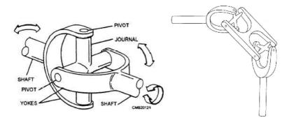
Figure 2.2.2-simple universal joint (left) and the double Cardan's joint concept (right)
