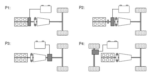
Figure 2.1.3 - Parallel hybrid powertrain distinction depending on the EM position (6)
