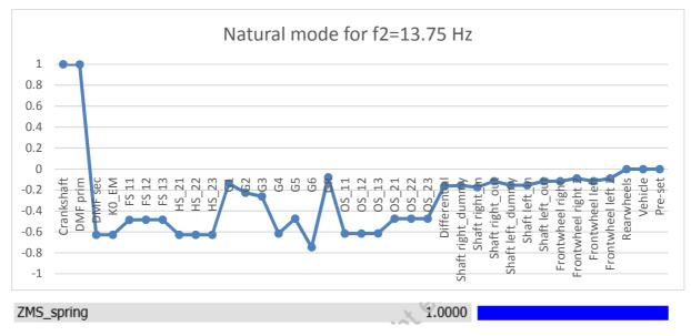
Figure 5.3.2 - f2 - DMF natural mode (top), potential energy (bottom)
