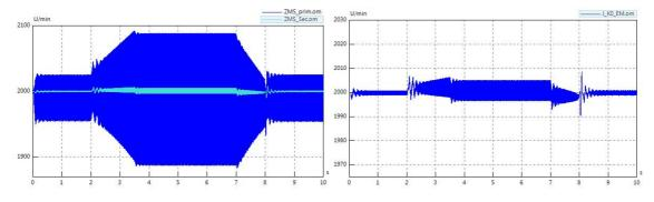
Figure 5.4.10 – Cycling 4<sup>th</sup> gear - angular velocity at the DMF primary side and secondary side (left) and clutch (right)
