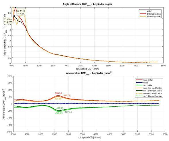
*Figure 6.4.7 - Comparison of the angle difference (top) and acceleration (bottom) for the DMF sec. inertia - initial vs. 3rd and 4th modification- 4-cylinder activated*
