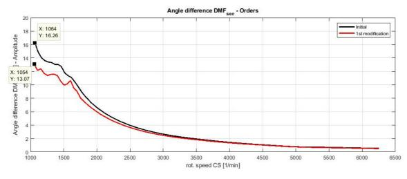
Figure 6.2.2 – Angle difference of the DMF sec. inertia with one stage DMF k=3 Nm/°
