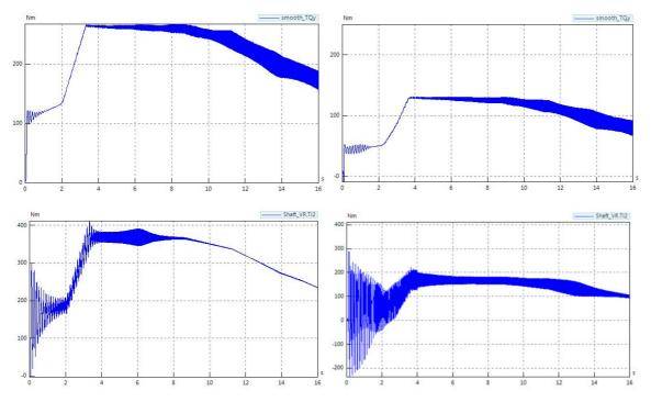
Figure 6.1.5 - Comparison engine torque (top) and right side shaft torque (bottom) for 4-cylinder (left) and 2-cylinder (right) activation
