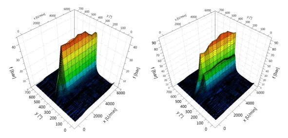
*Figure 5.2.6 - Engine pressure characteristic – zero load (left), full load (right)*
