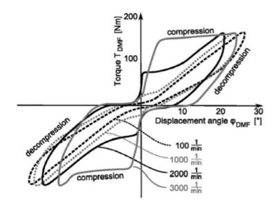
Figure 3.2.2 – Torsion at different engine speeds (16)
