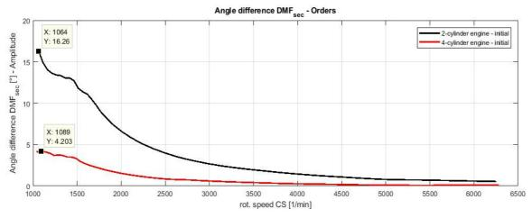
Figure 6.1.3 - 5th gear angle difference amplitude comparison for 2-cylinder and 4-cylinder activation
