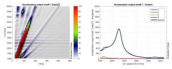
Figure 5.4.19 – 5<sup>th</sup> gear full load Campbell diagram (left) order analysis (right)
