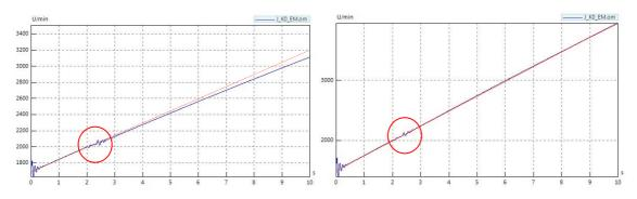
Figure 5.4.6 - Electric motor angular velocity for 0 Nm (left) and 15 Nm (right) torque increase during clutch closure
