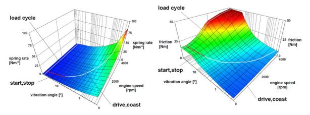
Figure 3.2.3 - Spring rate (left) and friction damping (right) as function of engine speed and vibration angle for a 2.51 diesel (17)
