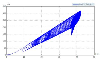
Figure 6.3.1 - Initial state DMF characteristic for 4-cylinder engine
