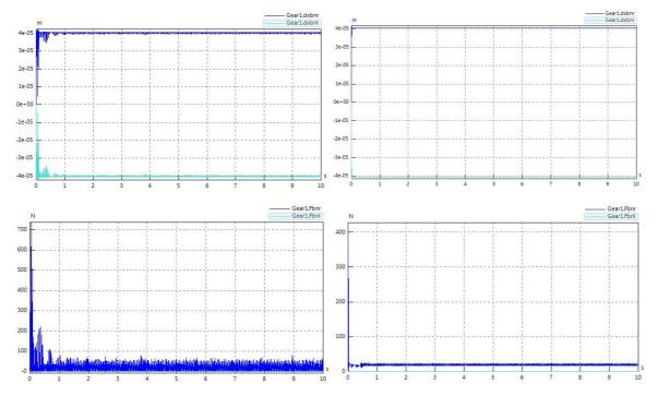
Figure 5.4.1 - Position difference and normal tooth flank force without DMF (left) and with DMF (right)
