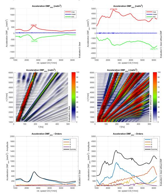
Comparison of run-up simulation in 5<sup>th</sup> gear of powertrain with and without DMF.
