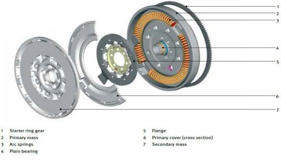
Figure 2.3.3- Components of a standard DMF
