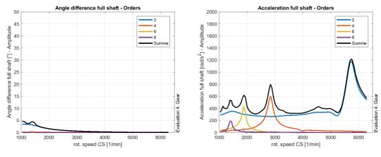
Figure 5.4.15 - 4th gear full load order analysis
