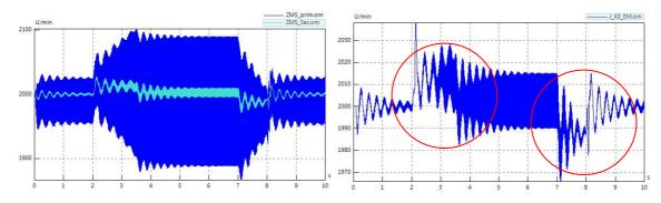
Figure 5.4.8 - Cycling 2<sup>nd</sup> gear - angular velocity at the DMF primary side and secondary side (left) and clutch (right)
