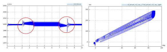
Figure 5.4.11 - Cycling 5th gear – clutch angular velocity (left) and DMF characteristic curve (right) with c<sub>2</sub>=3Nm/deg
