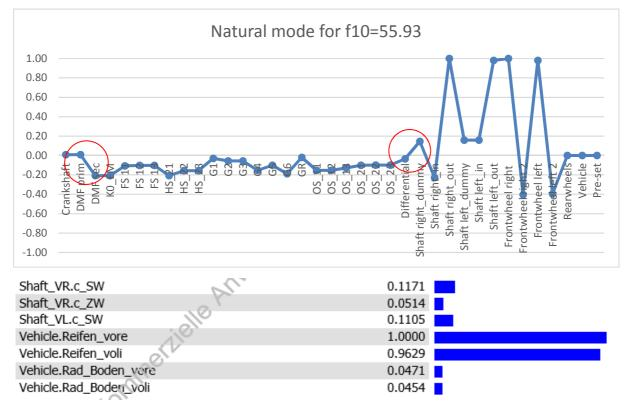
Figure 5.3.6 – f10 - Lower differential natural mode (top), potential energy (bottom)
