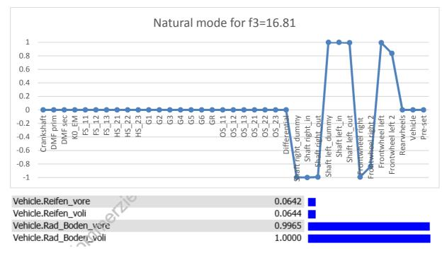
Figure 5.3.3 - f3 – side shafts and wheels twist against each other (top), potential energy (bottom)
