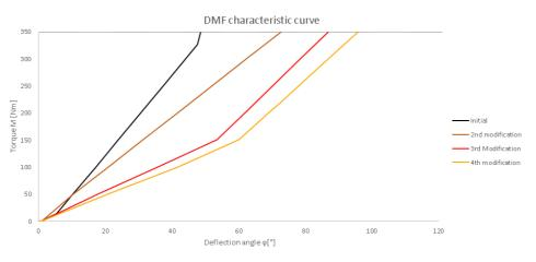
Figure 6.4.5 - DMF characteristic curve the initial state and all modifications
