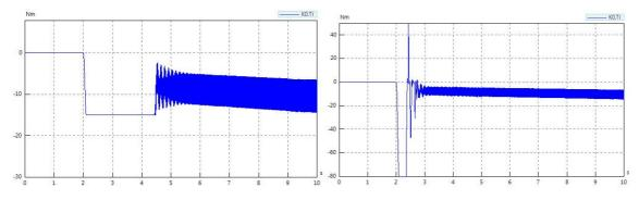
Figure 5.4.3 - Clutch torque withdrawal for 15 Nm (left) and 80 Nm (right)
