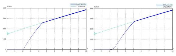
Figure 5.4.4 - Electric motor (light blue) and DMF secondary side (dark blue) angular velocity with 0.1 s (left) and 1 s (right) clutch closing time
