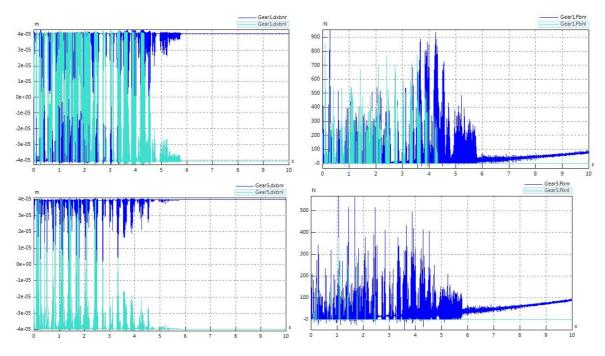
Figure 5.4.22 - Position difference (left) and normal tooth flank force (right) for the 1st gear pair (top) and 5th gear pair (bottom)
