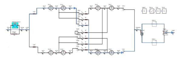
Figure 5.4.17 - Fifth gear power path
