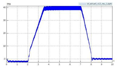
Figure 5.4.7 - Cycling - angle difference DMF arc spring – second gear
