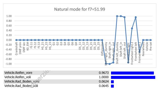
Figure 5.3.5 – f7 - Right and left side shaft and wheels twist against each other(top), potential energy (bottom)
