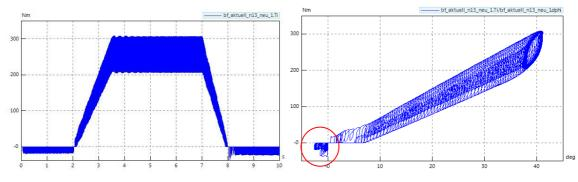
Figure 5.4.9 - Cycling 2<sup>nd</sup> gear - DMF torque (left) and DMF characteristic curve (right)
