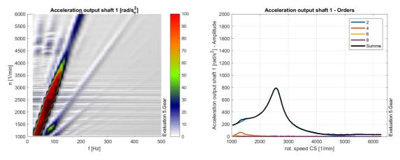
Figure 5.4.20 – 5<sup>th</sup> gear part load Campbell diagram (left) order analysis (right)
