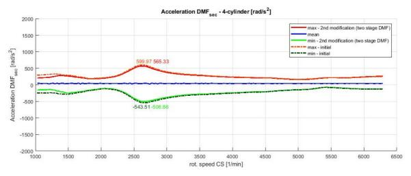
Figure 6.4.4 - Comparison of the acceleration for the DMF sec. inertia - initial vs. 2<sup>nd</sup> modification – 4-cylinder activated
