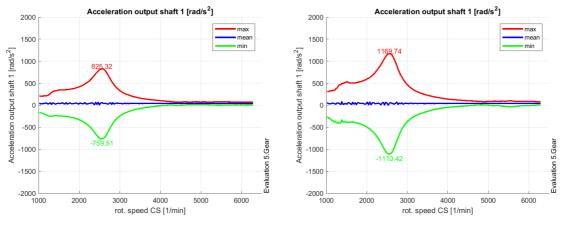
Figure 5.4.21 – 5<sup>th</sup> gear amplitude - part load (left) vs. full load (right)
