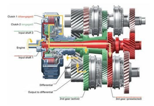
Figure 5.2.5 - dual-clutch transmission with selected 2nd gear (27)
