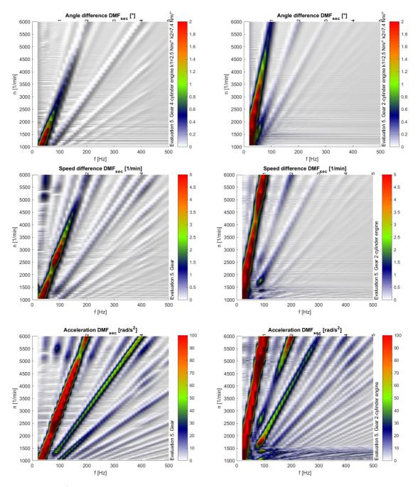
*Figure 6.1.2 – 5<sup>th</sup> gear comparison of angle, velocity and acceleration Campbell diagram for 4-cylinder activation (left) and 2-cylinder activation (right)*
