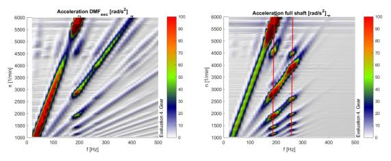
Figure 5.4.16 - 4th gear part load Campbell diagram - DMF (left), full shaft (right)
