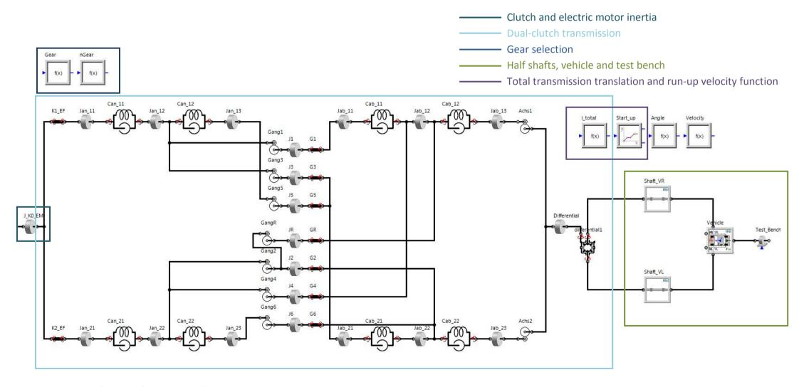
Figure 5.2.4 - MBS simulation model - transmission side
