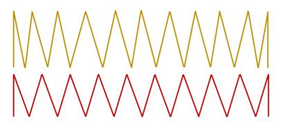
Figure 2.3.7 - Stage 1 torque reached -> spring 1 (yellow) has same length as spring 2 (red), when torque increases spring 1 and 2 start to deflect equally
