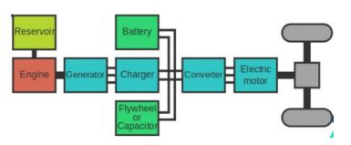
Figure 2.1.1- Series hybrid transmission scheme
