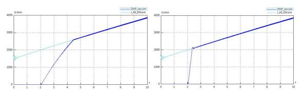
Figure 5.4.2 - Electric motor (light blue) and DMF secondary side (dark blue) angular velocity with 15 Nm (left) and 80 Nm (right) clutch torque
