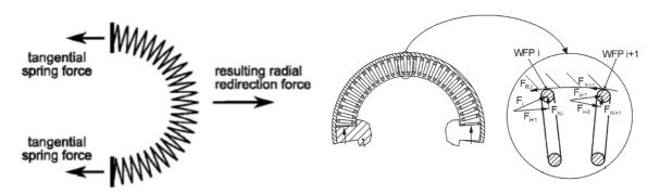
Figure 3.2.1 – Radial forces acting on the spring guides (left) (16) and forces acting on spring coils and absorption areas (WFP) (right)
