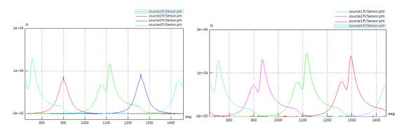
Figure 6.1.1 - Forces acting on the pistons for 2-cylinder activation (left) and 4-cylinder activation (right)
