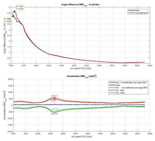
Figure 6.3.4- Comparison of the angle difference (top) and acceleration (bottom) for initial state vs. 1st modification (one stage DMF)
