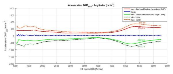
Figure 6.4.3 - Comparison of the acceleration for the DMF sec. inertia - initial vs. 2<sup>nd</sup> modification – 2-cylinder activated
