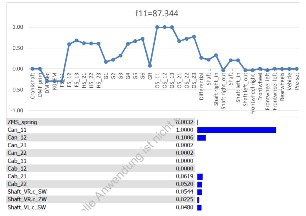
Figure 5.4.18 - Deflection and potential energy (5th gear)
