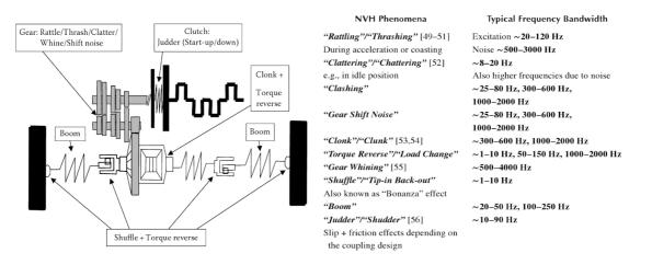
Figure 4.2 - NVH phenomena in a passenger car powertrain (FWD-left)) and their characteristic frequencies (right) (21)
