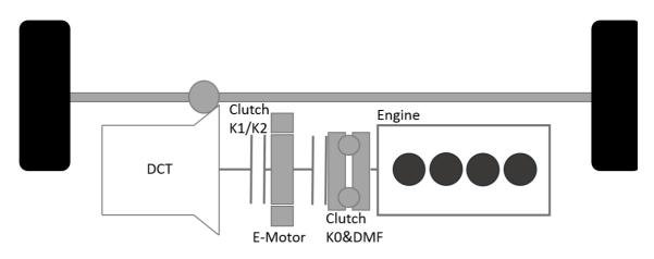
Figure 5.2.1 - P2 hybrid arrangement
