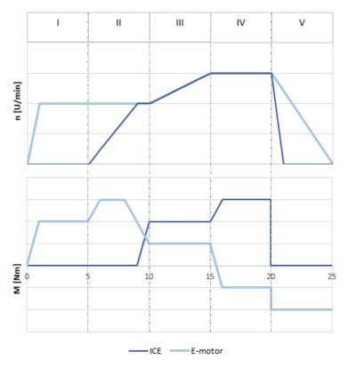
Figure 4.1.1 - Rotational speed and torque in hybrid specific operating conditions
