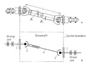
Figure 2.2.1 - Hooke's jointed shaft in a Z-configuration and diagrammatic representation of the system elements
