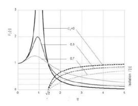
Figure 4.1.2 - Ideal isolation for different damping values ( $V_2$ =amplification function,  $\eta$ =frequency ratio)
