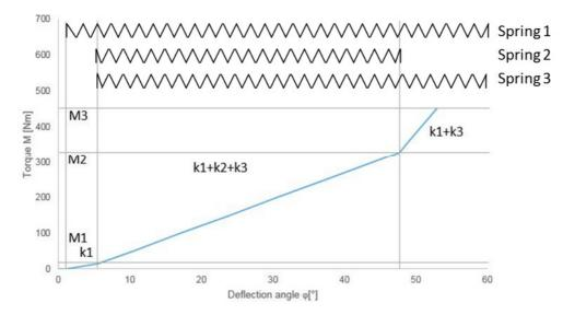
Figure 3.2.6 - DMF characteristic curve
