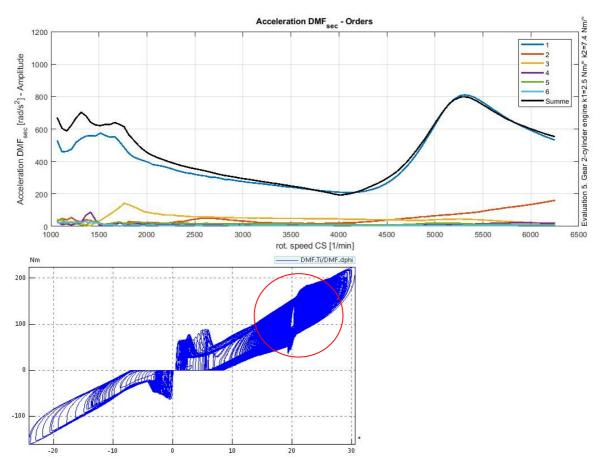
*Figure 6.1.4 – 2-cylinder activation order analysis (top) of secondary inertia acceleration and DMF characteristic curve for initial values (bottom) 5<sup>th</sup> gear*
