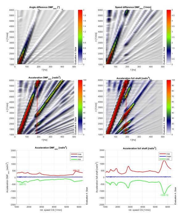
Figure 5.4.14 - 4th gear full load Campbell diagram (top and middle) for DMF secondary side angle difference (top - left), speed difference (top - right), acceleration (middle – left); full shaft acceleration (middle – right) and amplitude analysis (bottom) - DMF (left), full shaft (right)
