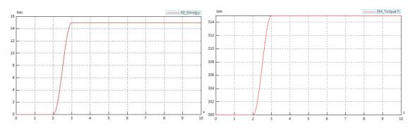
Figure 5.2.7 - Clutch torque (left) and electric motor torque (right) timing
