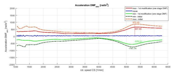
Figure 6.2.3 – Comparison of the acceleration of the DMF sec. inertia - initial DMF vs. one stage DMF with k=3 Nm/°
