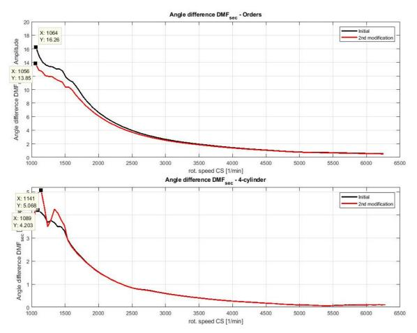
*Figure 6.4.2 – Comparison of the angle difference of the DMF sec. inertia for 2-cylinder (top) and 4-cylinder activation (bottom) - initial setting vs. 2<sup>nd</sup> modification*
