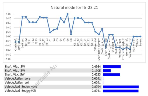
*Figure 5.3.4 – f6 - Wheels oscillate against transmission (top), potential energy (bottom)*
