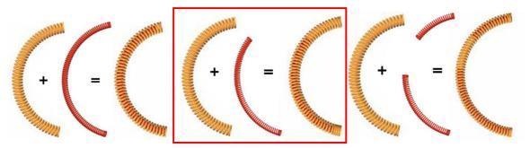
Figure 2.3.5 - From left: single-stage, two-stage and three-stage arc spring
