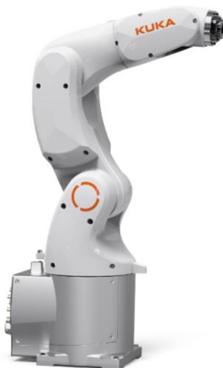
Obr. 5 – KUKA KR3 AGILUS [7]
