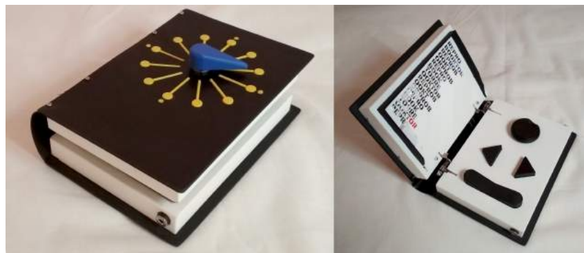
Figure 3.8: A 3D-printed prototype of Reprobooktor with tactile control elements. Two photos show the book closed (left) and opened (right). In the closed state, there is a handle that allows switching between particular book titles. The yellow circular buttons provide information about the book title. While opened, there are tactile controls that correspond to the description in Figure 3.4 above.
