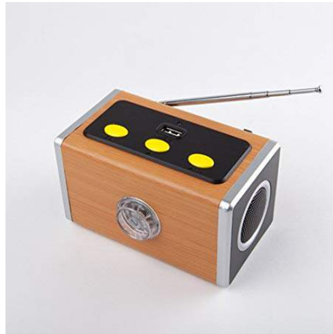
Figure 2.9: UI of BoomBox plus device, from [67]. The UI consist of there buttons and main ON/OFF switch. The ON/OFF is located on the back of the device. On the top of device are there identical buttons. The middle button covers the play/pause function, the others skip track (in the radio mode skip the station).
