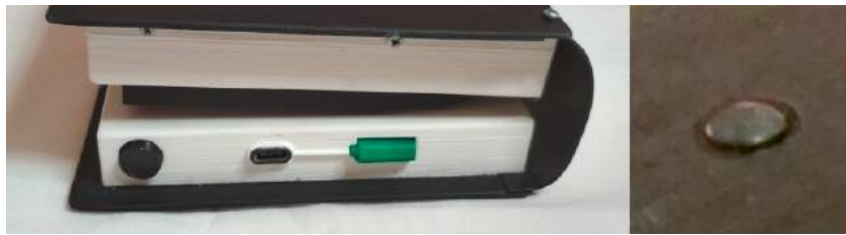
Figure 3.9: The left image shows the added battery status button, watch button, and power connector on the high-fidelity prototype. The right image shows the rubber leg.
