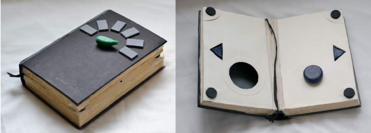
Figure 3.6: A physical prototype of Reproboktor with tactile control elements. Two photos show the book closed (left) and opened (right). In the closed state, there is a handle that allows switching between particular book titles. While opened, there are tactile controls that correspond to the description in Figure 3.3 above.
