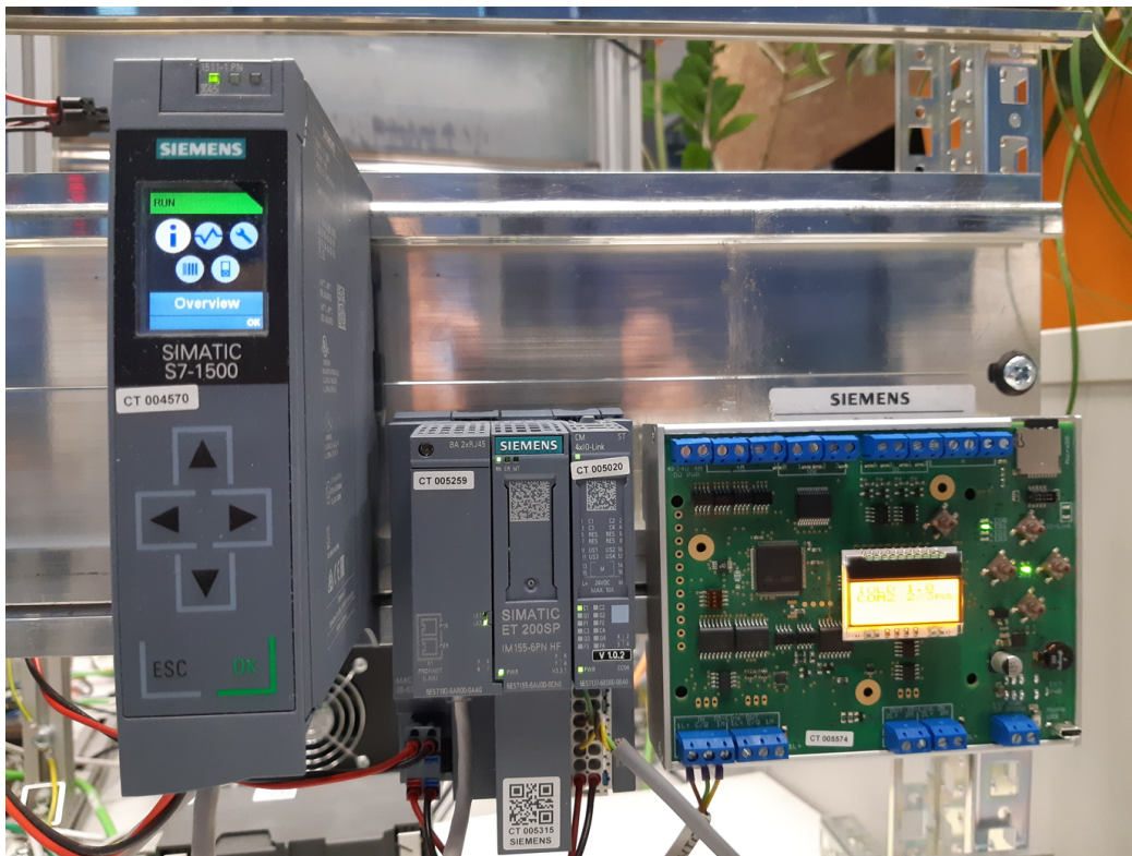
Figure 5.15: Proof of concept station: PLC on the left, IO-Link Master in the middle and the IOLTD on the right
