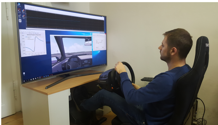
Figure 5.2: Virtual test driving. Testing the designed controller by virtual test driving on simulation platform that connects Simulink with IPG Carmaker and steering wheel.
